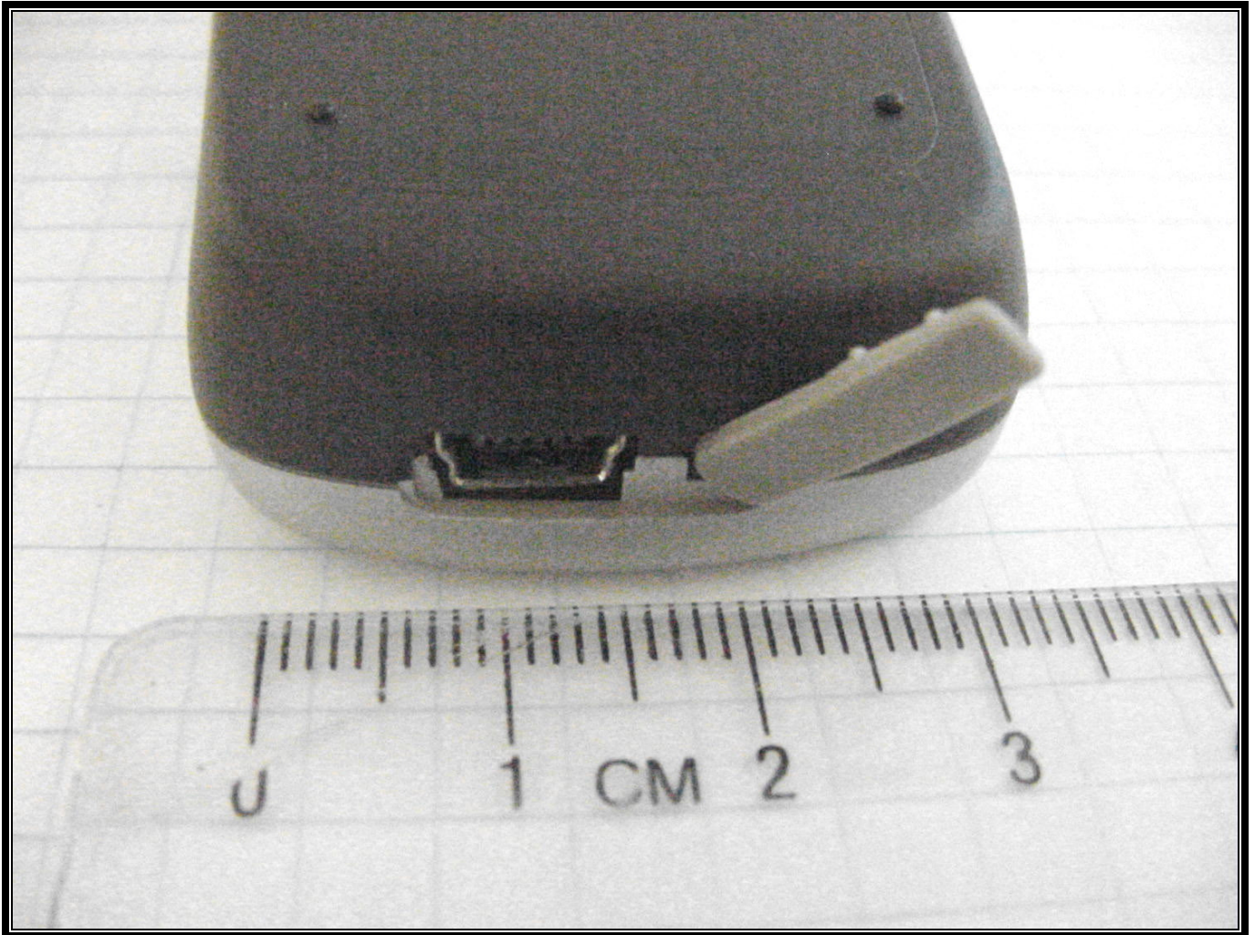
PHOTOGRAPH 7: BOTTOM VIEW SHOWING RECHARGE CONNECTOR
