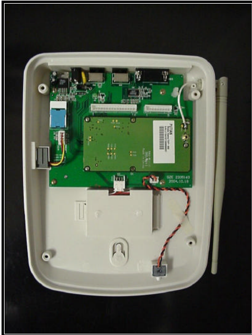
PHOTOGRAPH 22: RF AND MAIN PCB'S MOUNTED IN CHASSIS
