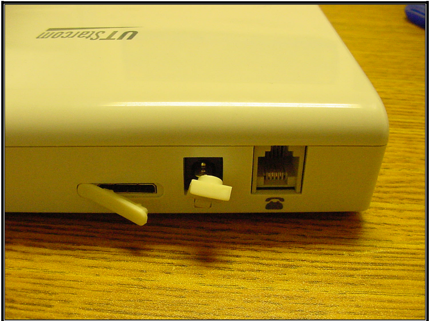
PHOTOGRAPH 11: REAR VIEW SHOWING POWER, RJ-11 AND DATA CONNECTIONS
