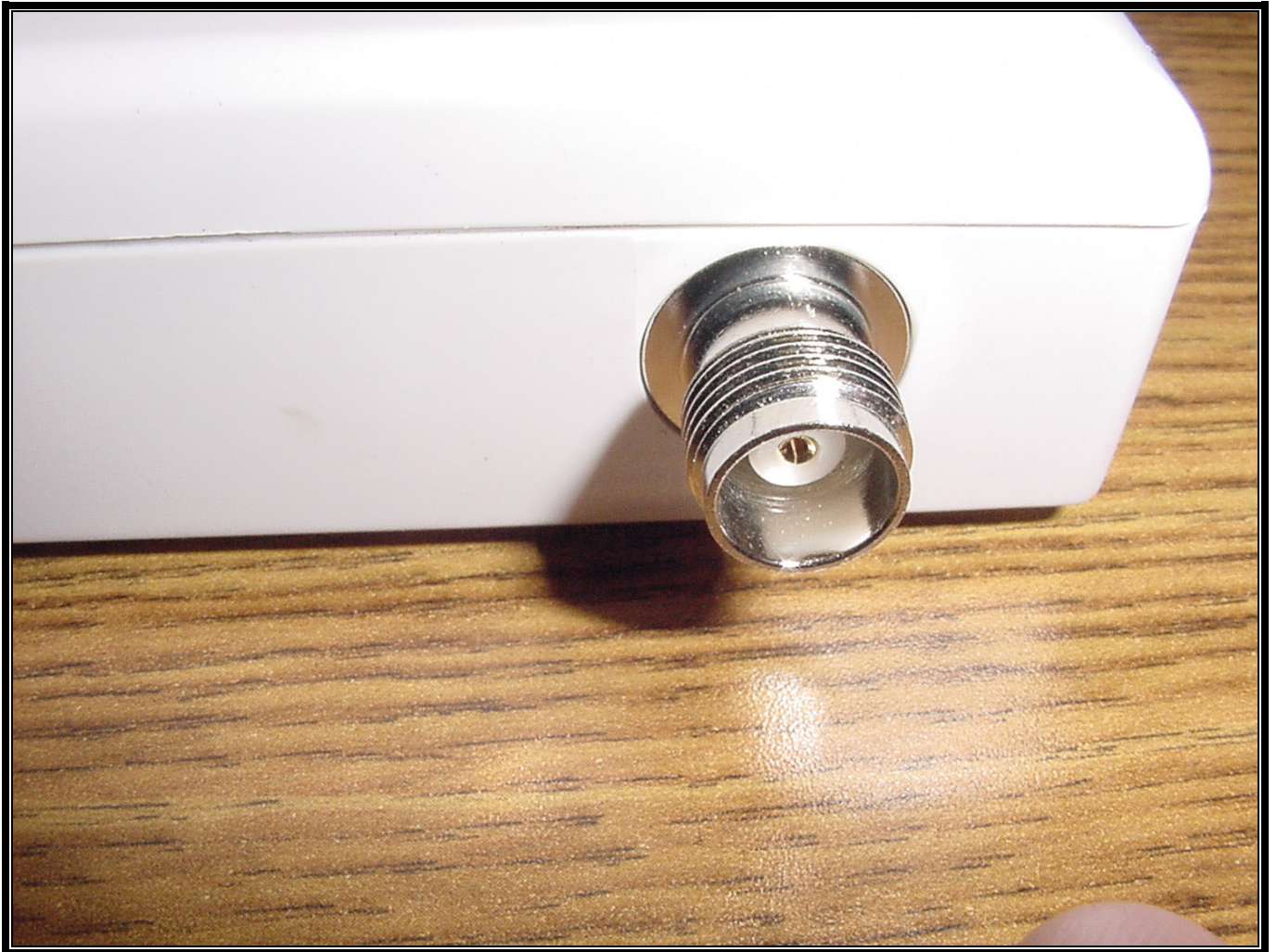
PHOTOGRAPH 10: RIGHT SIDE VIEW SHOWING ANTENNA CONNECTOR
