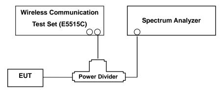
(Configuration of conducted Emission measurement)
