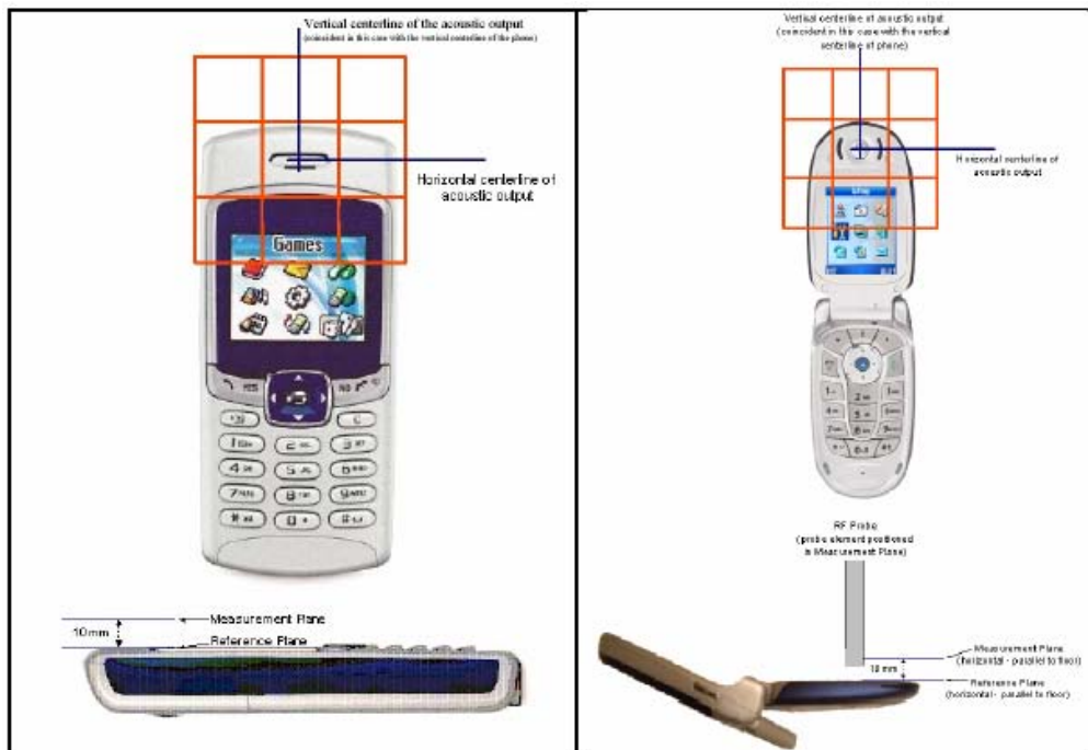
Figure 3. WD reference and plane for RF emission measurements
