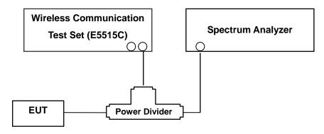
(Configuration of conducted Emission measurement)
