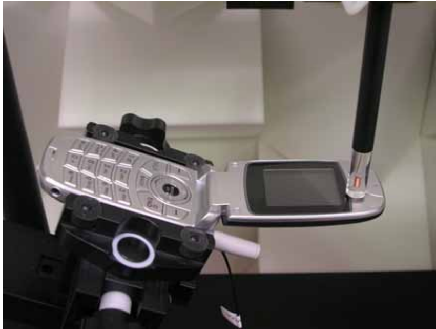
Figure 13-1 Test Setup for Wireless Device
