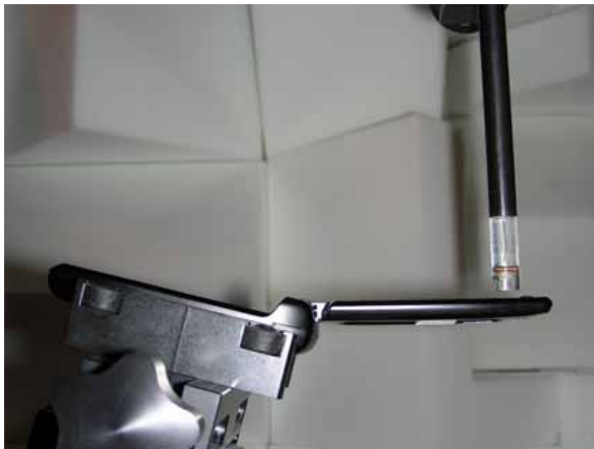
Figure 13-2 Test Setup for Wireless Device
