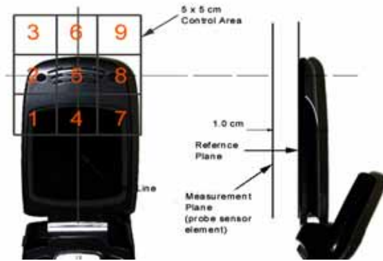
Figure 13 E/H-Field Emissions Test Setup Diagram
