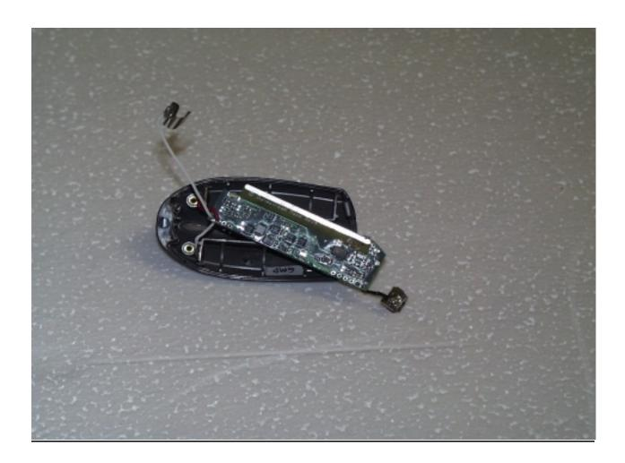
PRINTED CIRCUIT BOARD REMOVED (Rear View)
