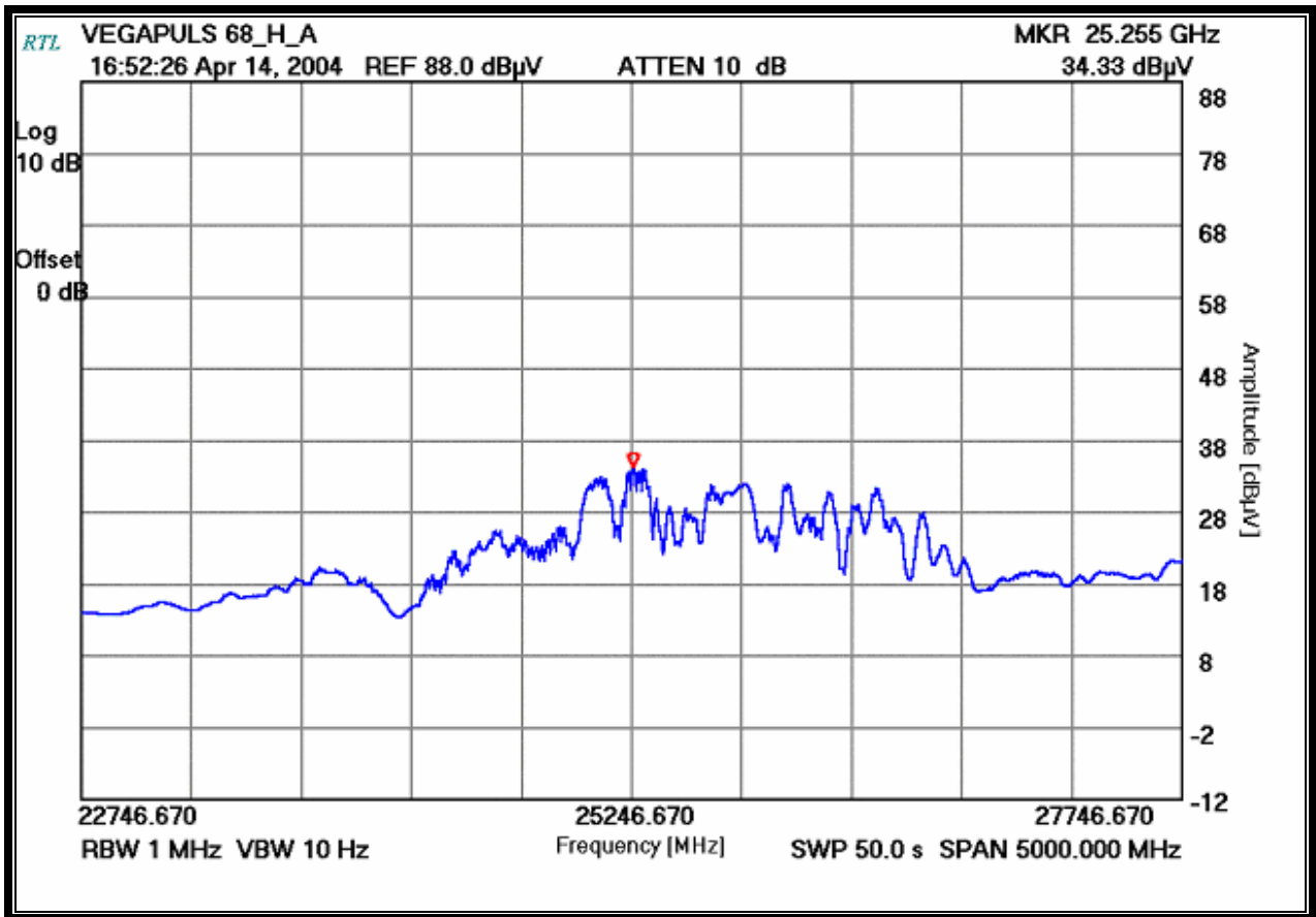
PLOT 6-3 EUT 19.5 DBI HORN ANTENNA 100% DUTY CYCLE AVERAGE MODE
