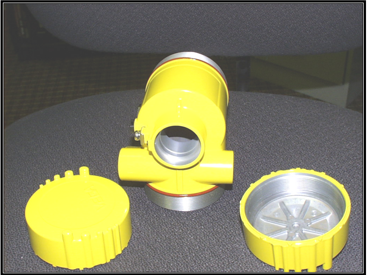
PHOTOGRAPH 11: EUT DOUBLE ALUMINUM CHAMBER HOUSING REAR VIEW
