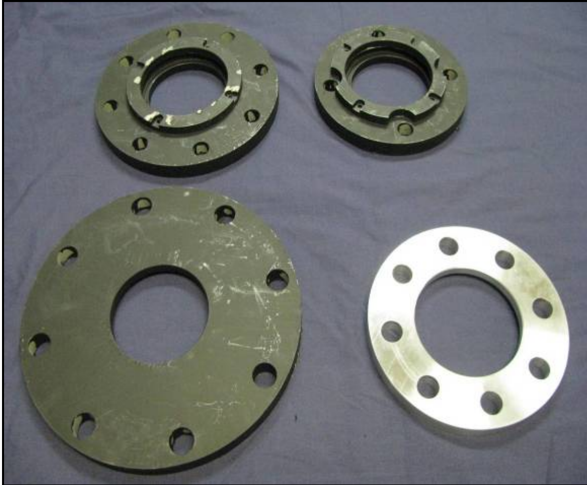
Photograph 11: Aluminum and Metalized Plastic Flanges
