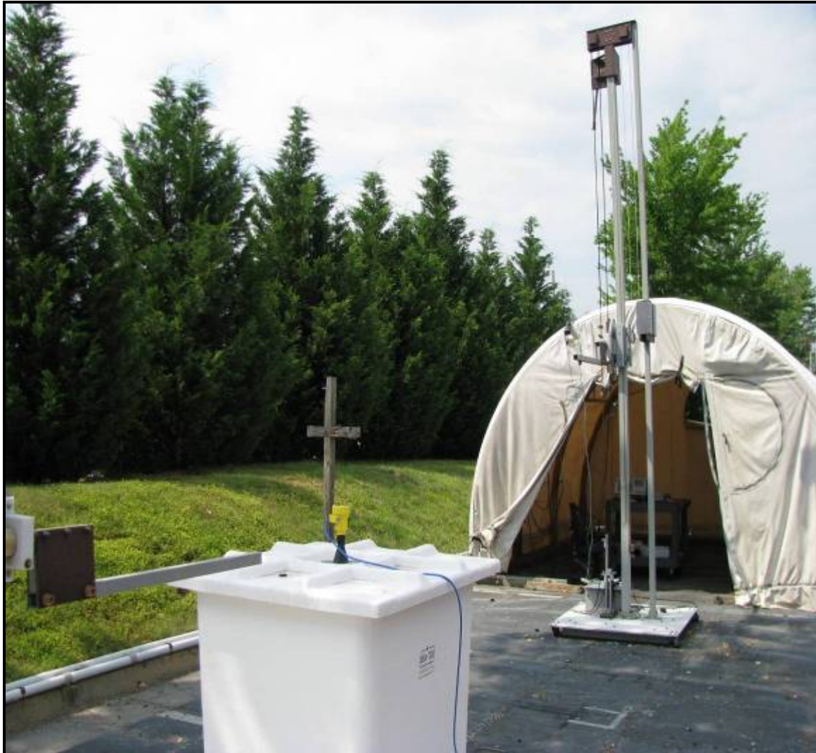
Photograph 4: Radiated Emissions - EUT in Fiberglass Tank
