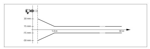
Fig. 34: Accuracy VEGAPULS 62 with horn antenna and increased sensitivity
