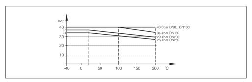
Fig. 39: DIN flange PN 40 temperature derating in bar/°C
