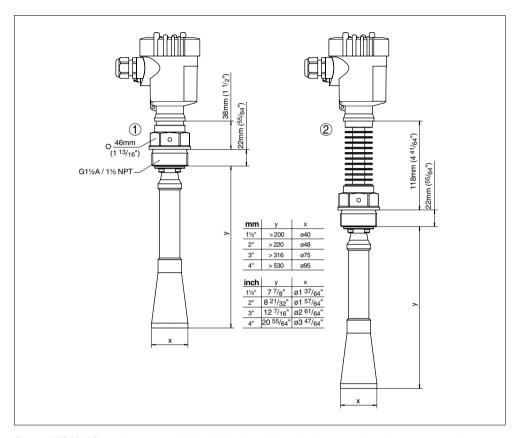
Fig. 57: VEGAPULS 62 - horn antenna in threaded version with purging air connection and antenna extension<sup>18)</sup>
