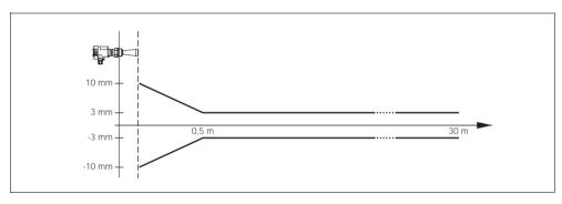
Fig. 33: Accuracy VEGAPULS 62 with horn antenna
