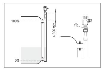
Fig. 15: VEGAPULS in a bypass tube
