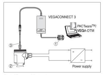
Fig. 31: PC connected directly to the sensor
