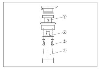
Fig. 4: Dismounting of the horn antenna
