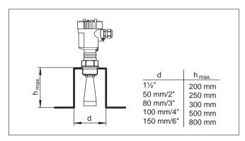
Fig. 10: Deviating socket dimensions
