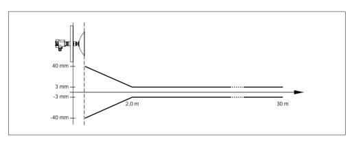
Fig. 35: Accuracy VEGAPULS 62 with parabolic antenna
