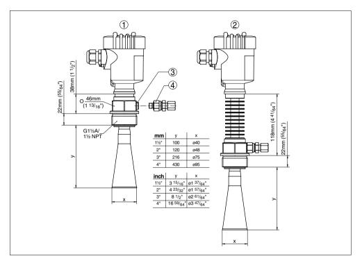
Fig. 56: VEGAPULS 62 - horn antenna in threaded version with rinsing air connection
