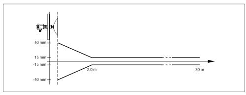
Fig. 36: Accuracy VEGAPULS 62 with parabolic antenna and increased sensitivity
