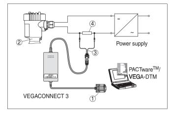
Fig. 32: Connecting the PC to the signal cable
