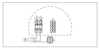
Fig. 23: Wiring plan, double chamber housing
