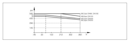
Fig. 40: DIN flange PN 40 temperature derating in psi/°F
