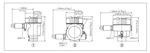
Fig. 54: Housing versions in protection IP 66/IP 68, 1 bar (with integrated PLICSCOM the housing is 9 mm/0.35 in higher)
