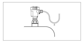
Fig. 2: Measures against moisture penetration
