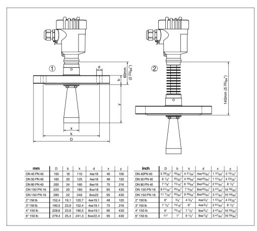
Fig. 58: VEGAPULS 62 - horn antenna in flange version
