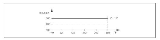
Fig. 46: ANSI flange 300 lbs temperature derating based on °F
