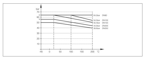
Fig. 41: DIN flange PN 64 temperature derating in bar/°C
