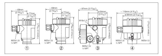
Fig. 53: Housing versions in protection IP 66/IP 67 and IP 66/IP 68, 0.2 bar (with integrated PLICSCOM the housing is 9 mm/0.35 in higher)
