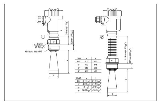
Fig. 55: VEGAPULS 62 - horn antenna in threaded version
