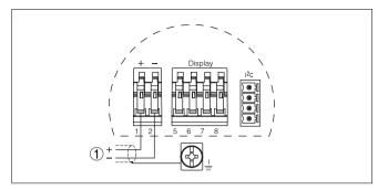
Fig. 19: Wiring plan, single chamber housing
