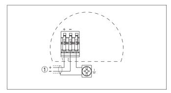
Fig. 27: Wiring plan, double chamber housing Exd 1 Power supply/Signal output
