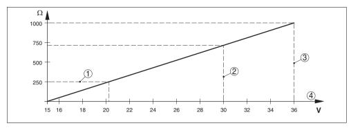
Fig. 52: Voltage diagram for version with increased sensitivity
