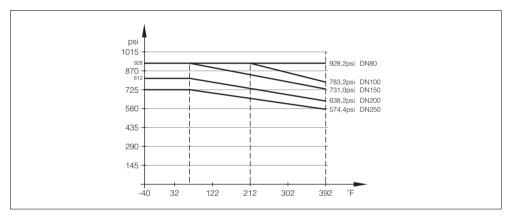
Fig. 42: DIN flange PN 64 temperature derating in psi/°F
