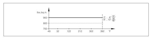
Fig. 50: ANSI flange 900 lbs temperature derating based on °F
