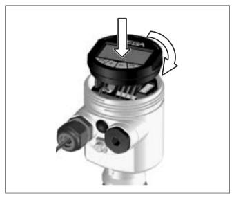
Fig. 29: Installation of PLICSCOM
