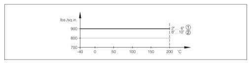
Fig. 49: ANSI flange 900 lbs temperature derating based on °C
