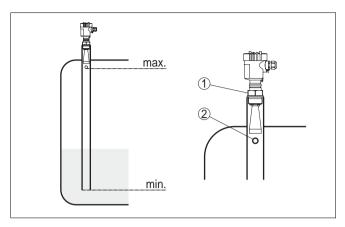
Fig. 14: Pipe antenna systems in a tank
