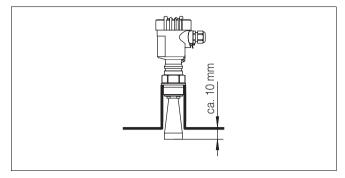
Fig. 9: Recommended socket mounting
