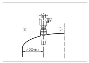
Fig. 6: Mounting on dished vessel tops
