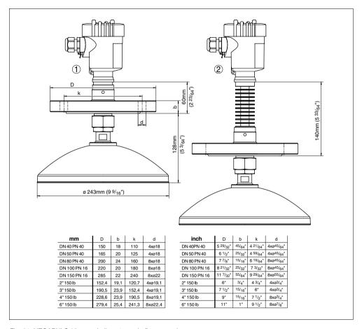
Fig. 61: VEGAPULS 62 - parabolic antenna in flange version
