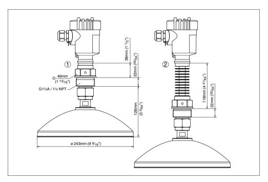
Fig. 60: VEGAPULS 62 - parabolic antenna in threaded version
