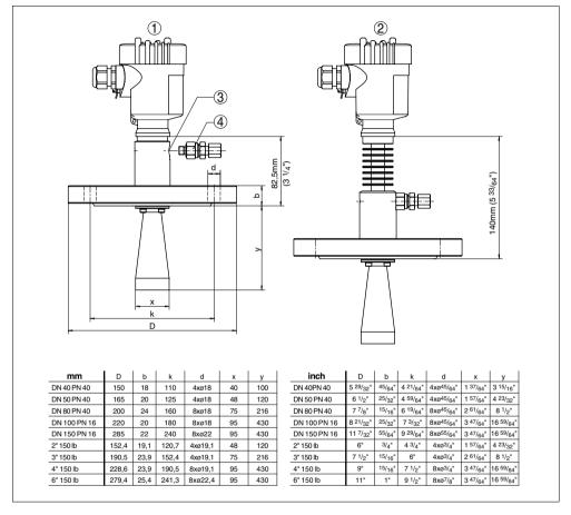
Fig. 59: VEGAPULS 62 - horn antenna in flange version with rinsing air connection
