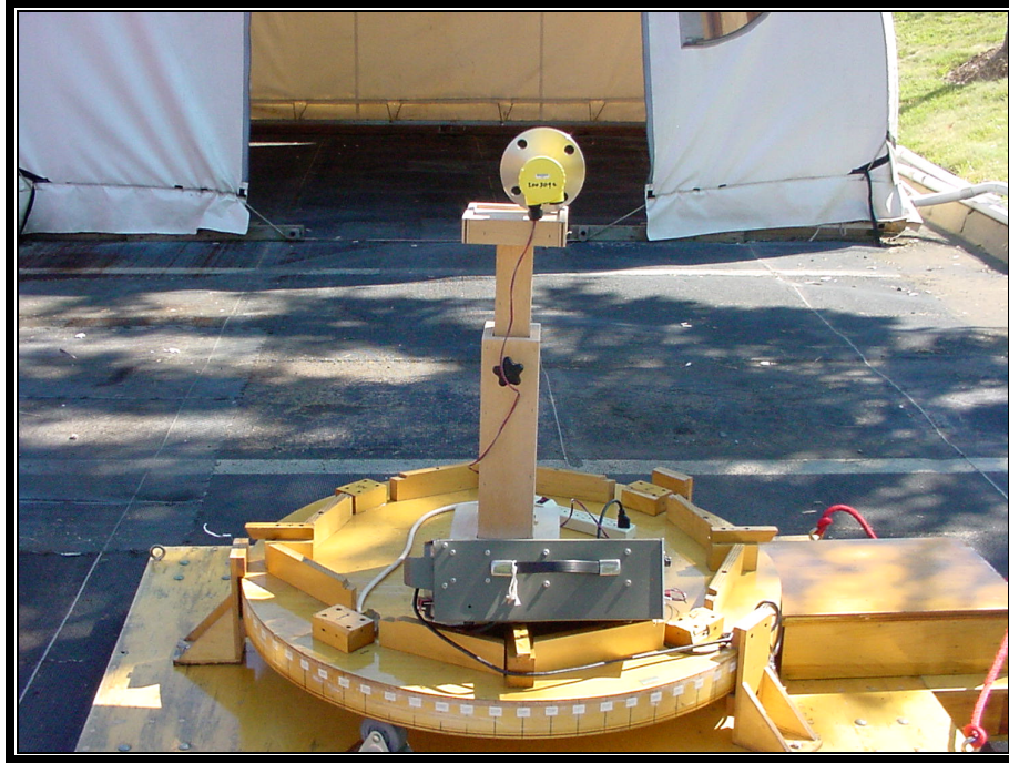
Photograph 15: Radiated Emissions Front View 21.2dBi Horn Antenna
