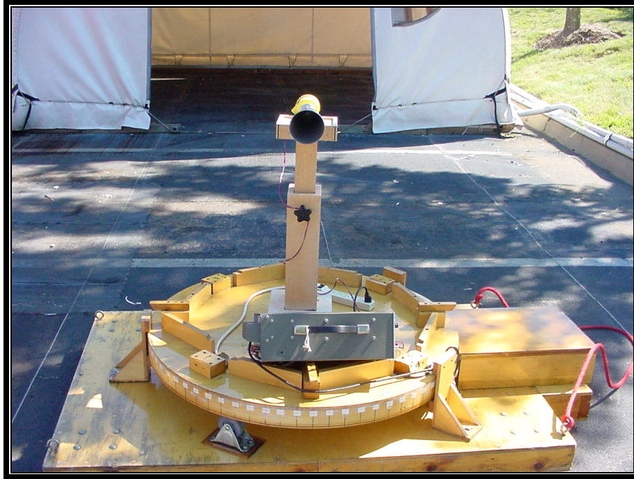
Photograph 14: Radiated Emissions Rear View 24.7dBi Horn Antenna
