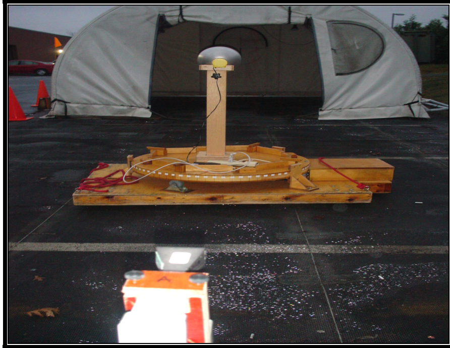
Photograph 8: Radiated Emissions Rear View 33 dBi Parabolic Antenna
