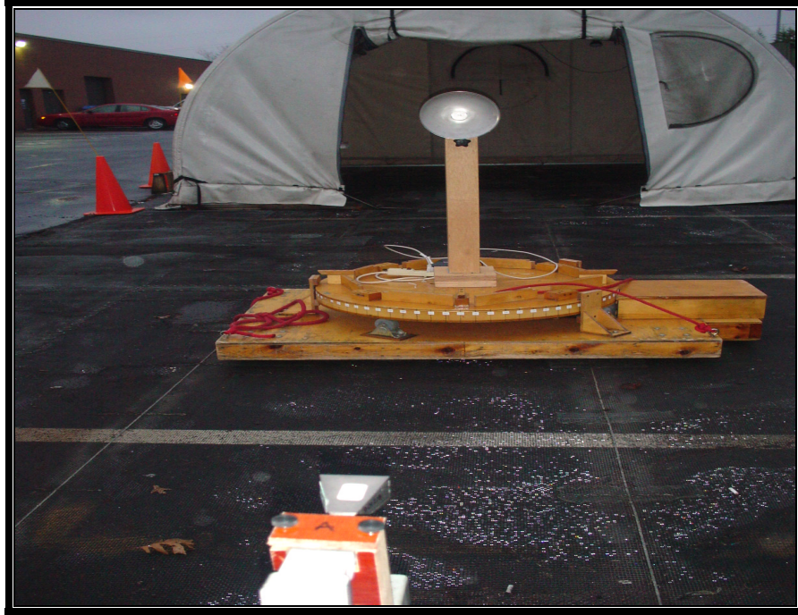
Photograph 7: Radiated Emissions Front View 33 dBi Parabolic Antenna
