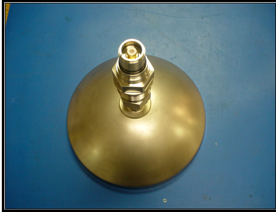
Photograph 38: 33 dBi Parabolic Antenna Top View
