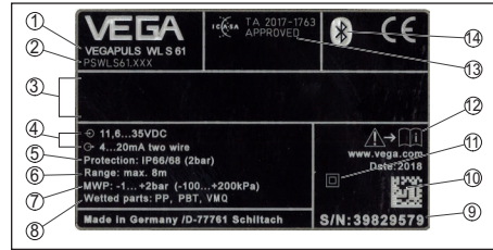
Abb. 17: Layout of the type label (example)
