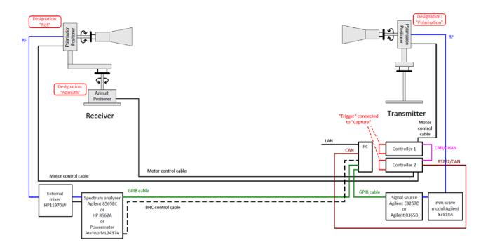
To determine the antenna gain the gain-transfer method (gain-comparison measurement) is used. First a standard gain horn is measured in the above described setup and the results recorded. Standard gain horn information:
