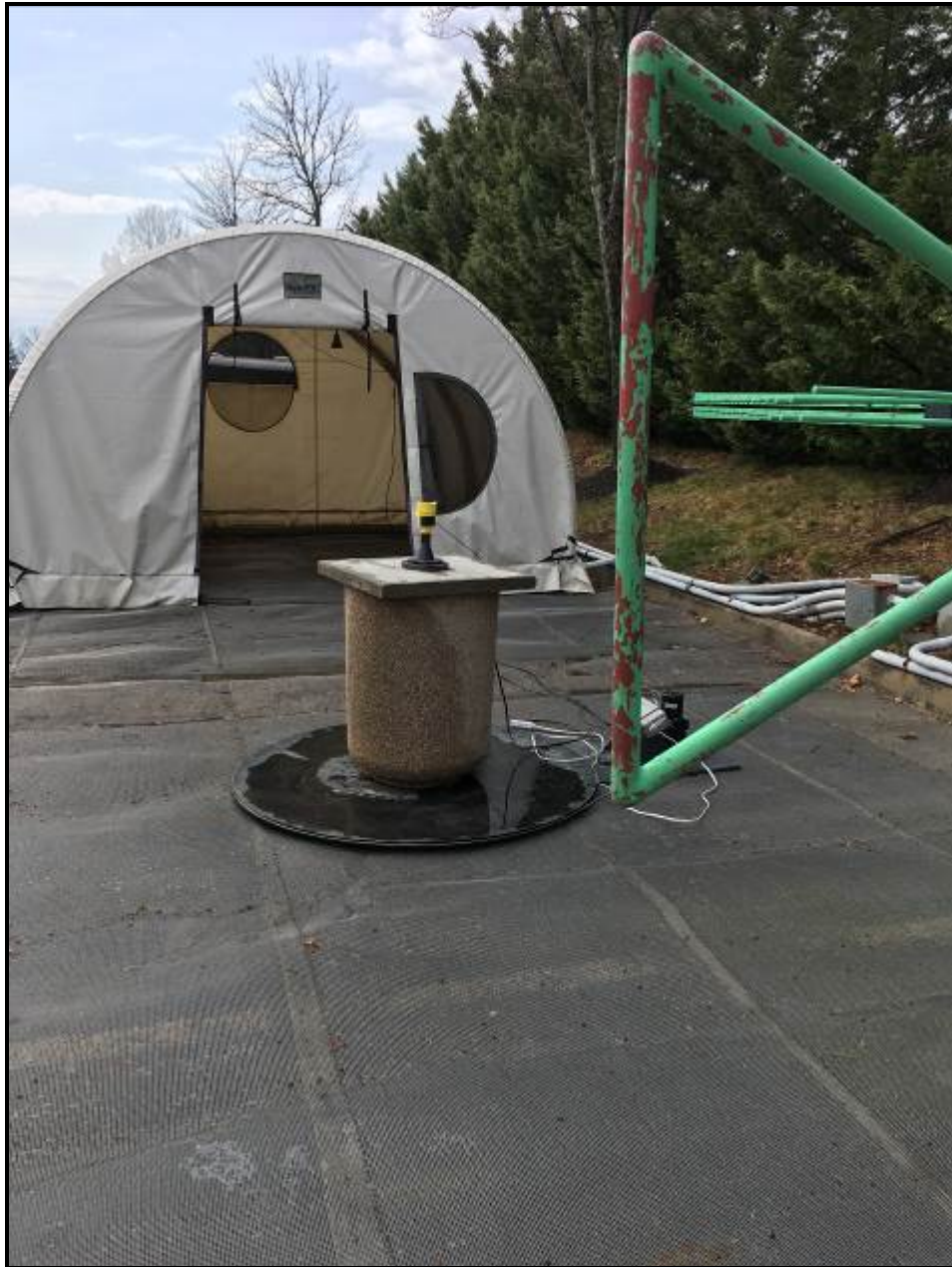
Photograph 11: Radiated Emissions – TC #1; Concrete Container
