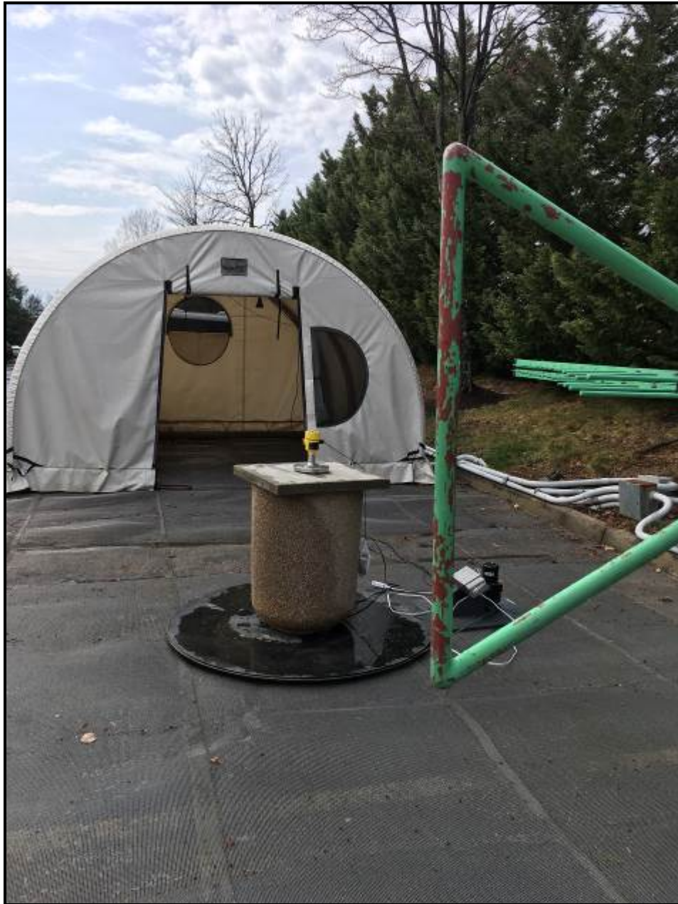
Photograph 14: Radiated Emissions – TC #2; Concrete Container
