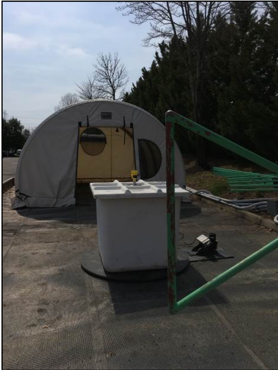
Photograph 16: Radiated Emissions – TC #2; Fiberglass Container
