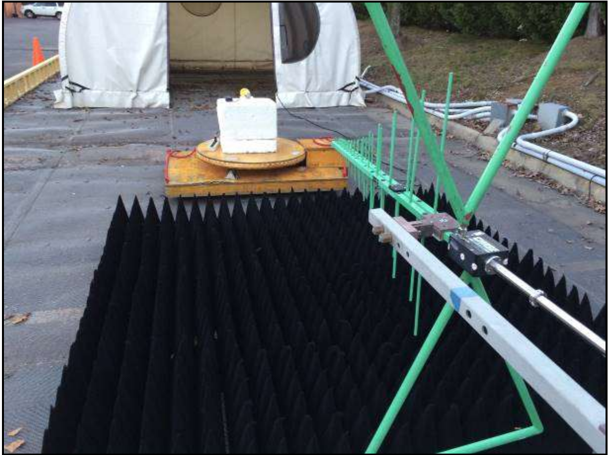
Photograph 4: Radiated Emissions – Typical View of Emissions Greater Than 1 GHz
