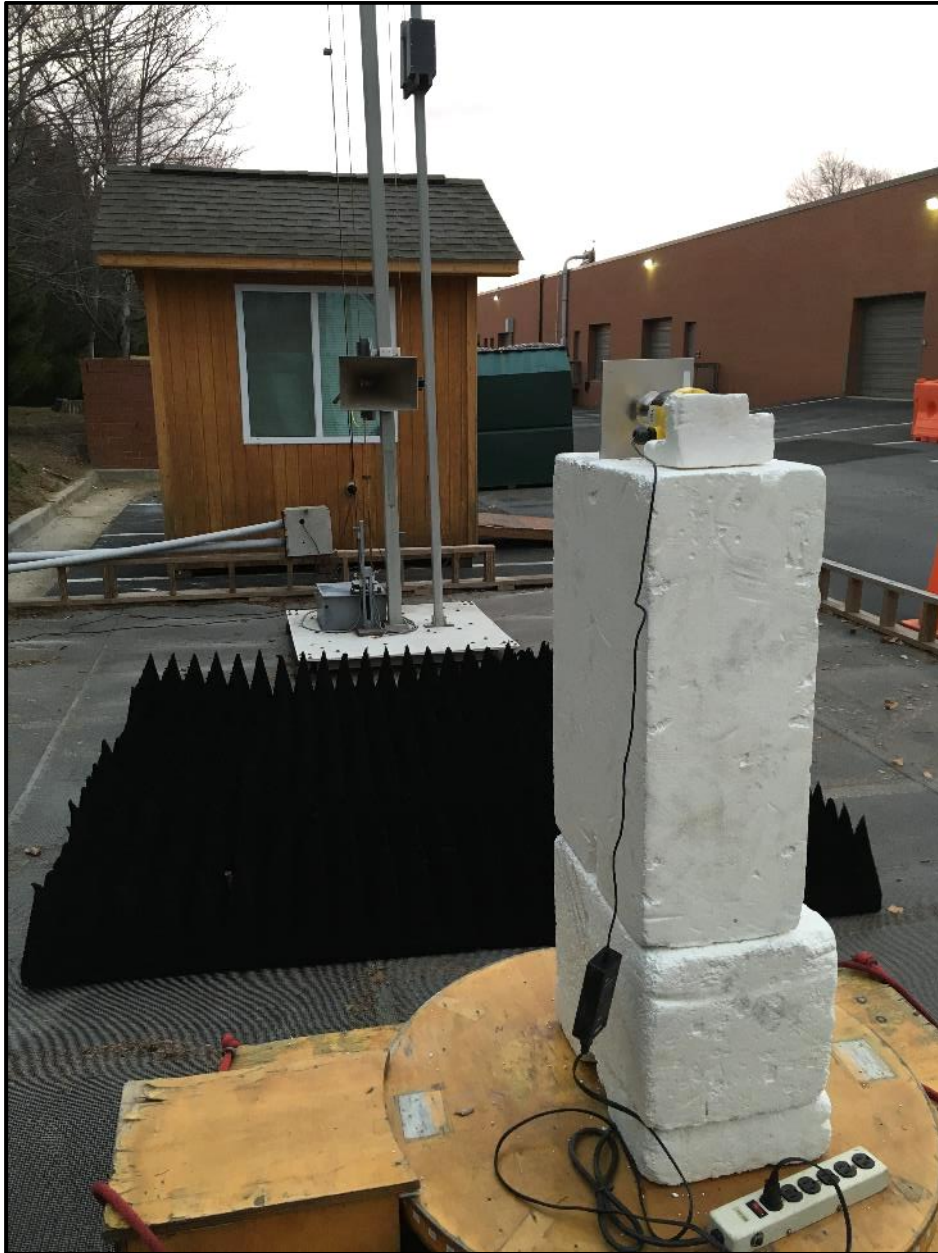
Photograph 5: Radiated Emissions – Rear View (>1 GHz)
