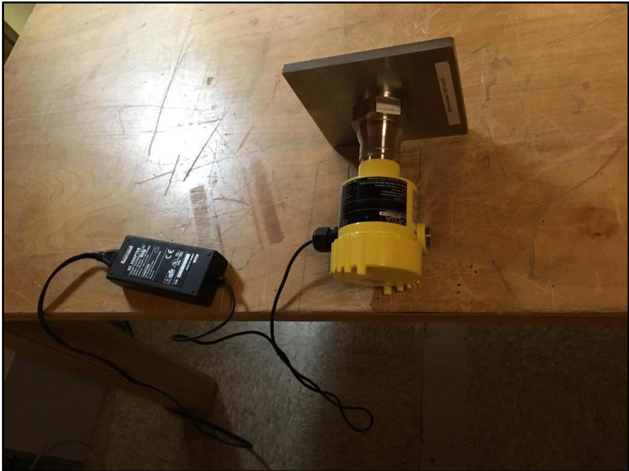
Photograph 7: AC Conducted Emissions - Rear View
