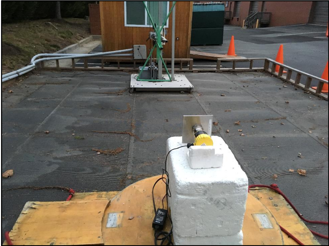
Photograph 3: Radiated Emissions – Rear View (<1 GHz)
