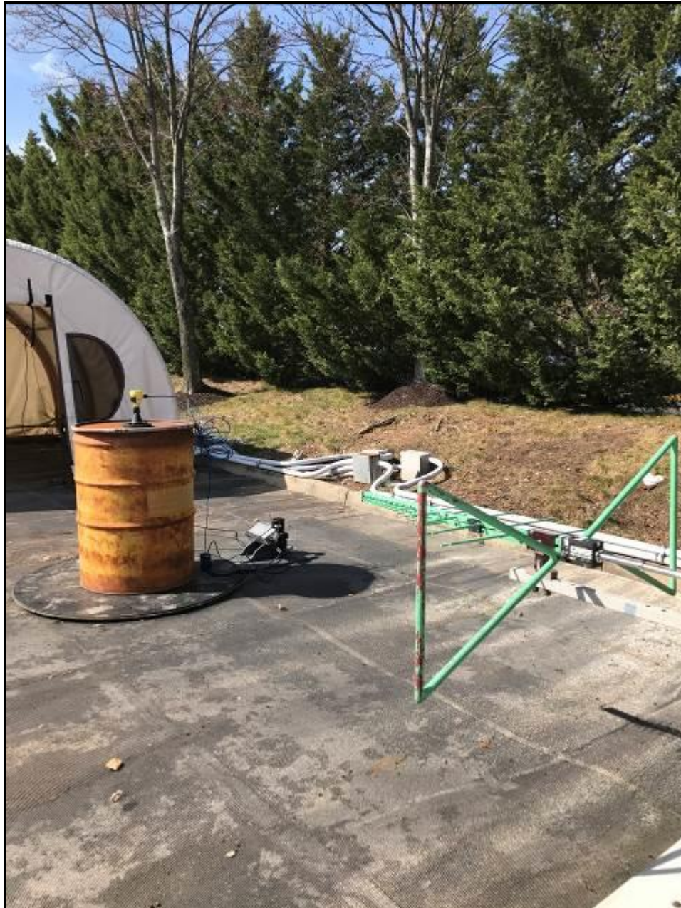
Photograph 12: Radiated Emissions – TC #1; Steel Container
