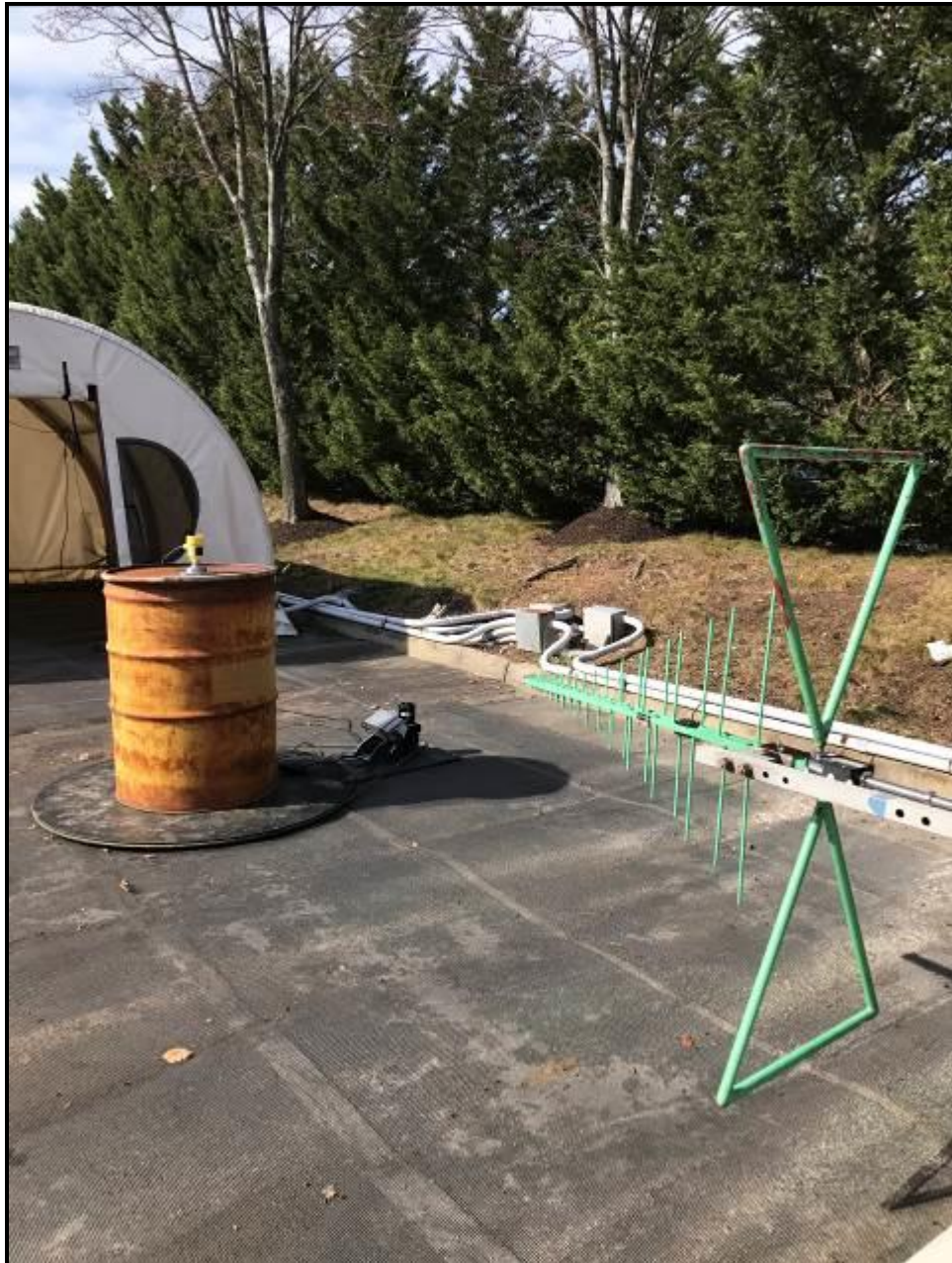
Photograph 15: Radiated Emissions – TC #2; Steel Container
