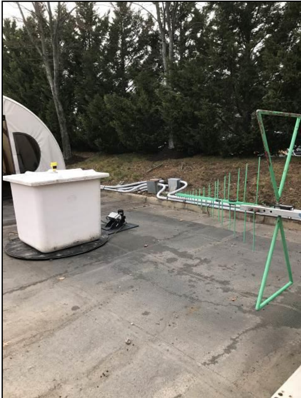
Photograph 16: Radiated Emissions – TC #2; Fiberglass Container
