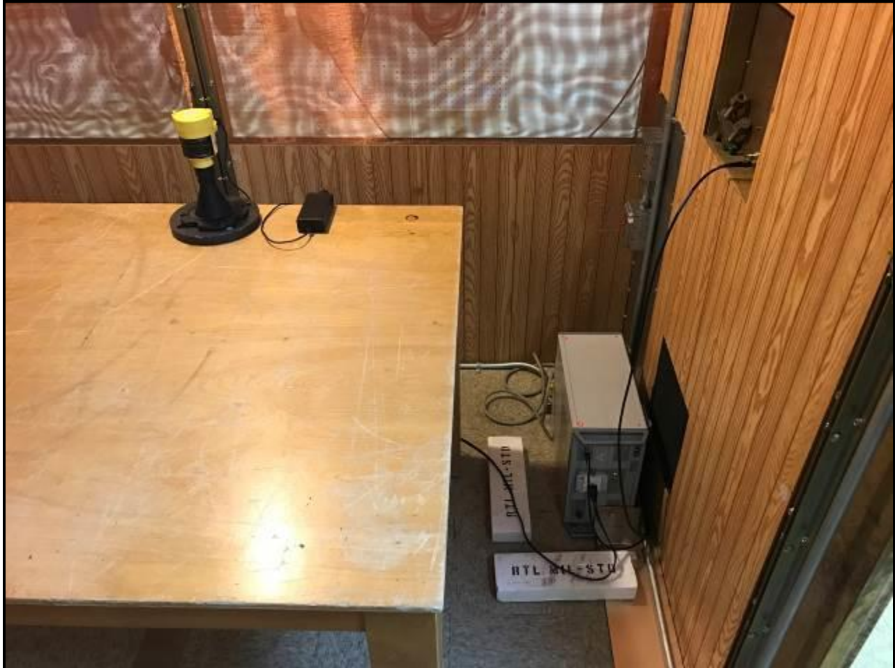
Photograph 5: AC Conducted Emissions – Front View - TC #1
