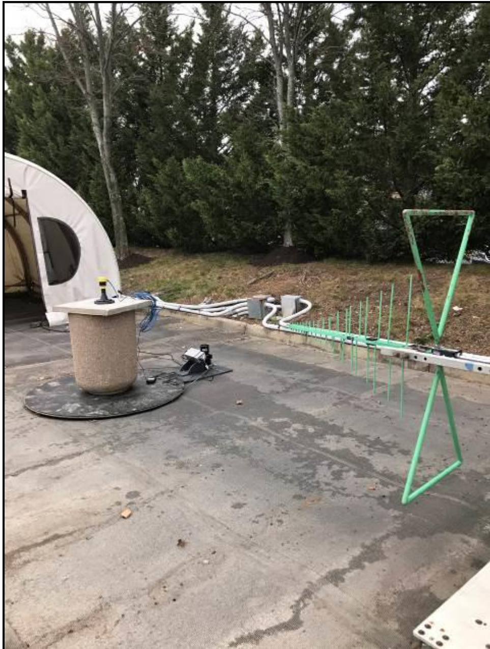
Photograph 11: Radiated Emissions – TC #1; Concrete Container
