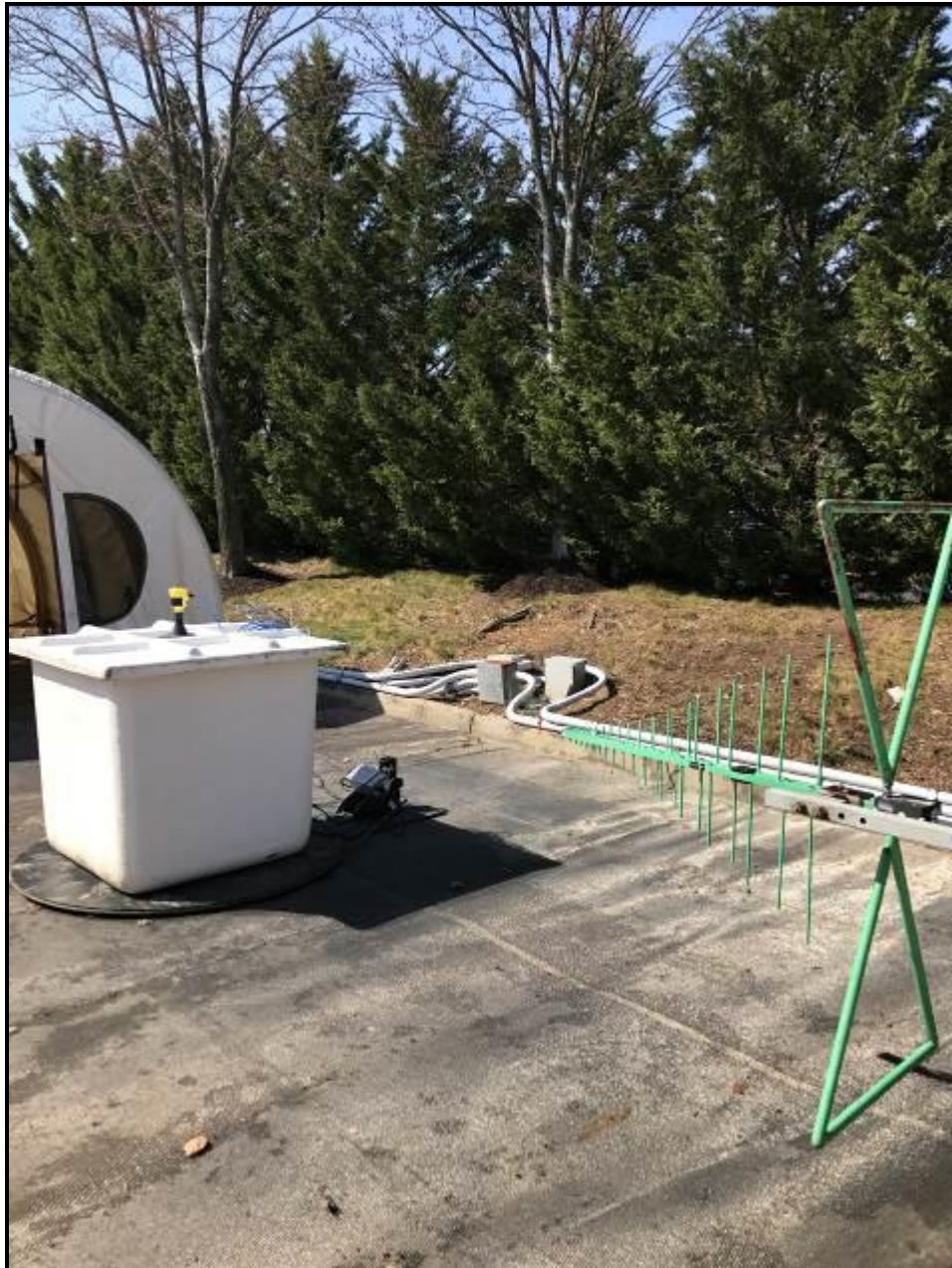
Photograph 13: Radiated Emissions – TC #1; Fiberglass Container
