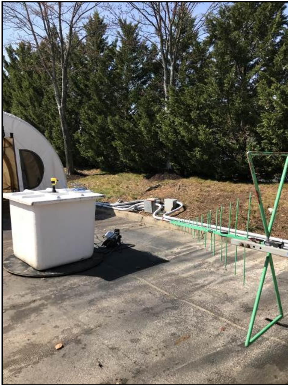
Photograph 13: Radiated Emissions – TC #1; Fiberglass Container
