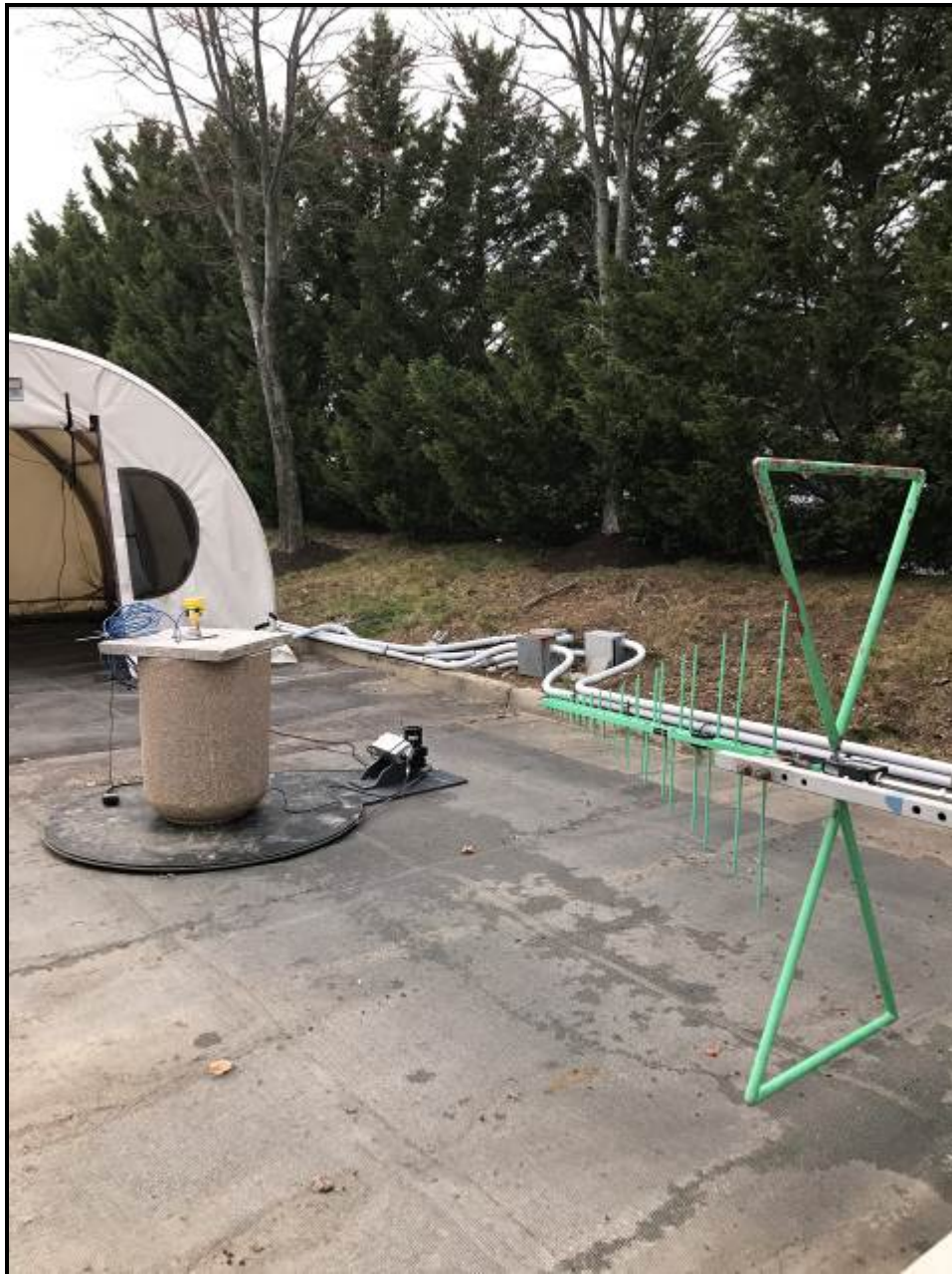
Photograph 17: Radiated Emissions – TC #3; Concrete Container
