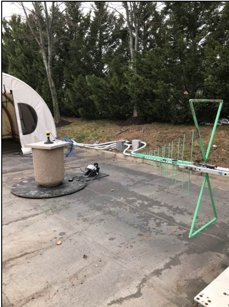
Photograph 11: Radiated Emissions – TC #1; Concrete Container
