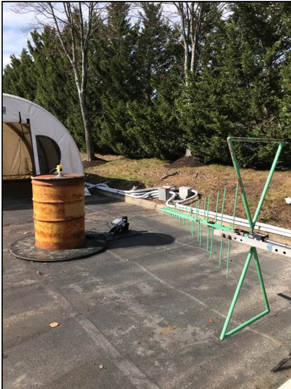
Photograph 15: Radiated Emissions – TC #2; Steel Container
