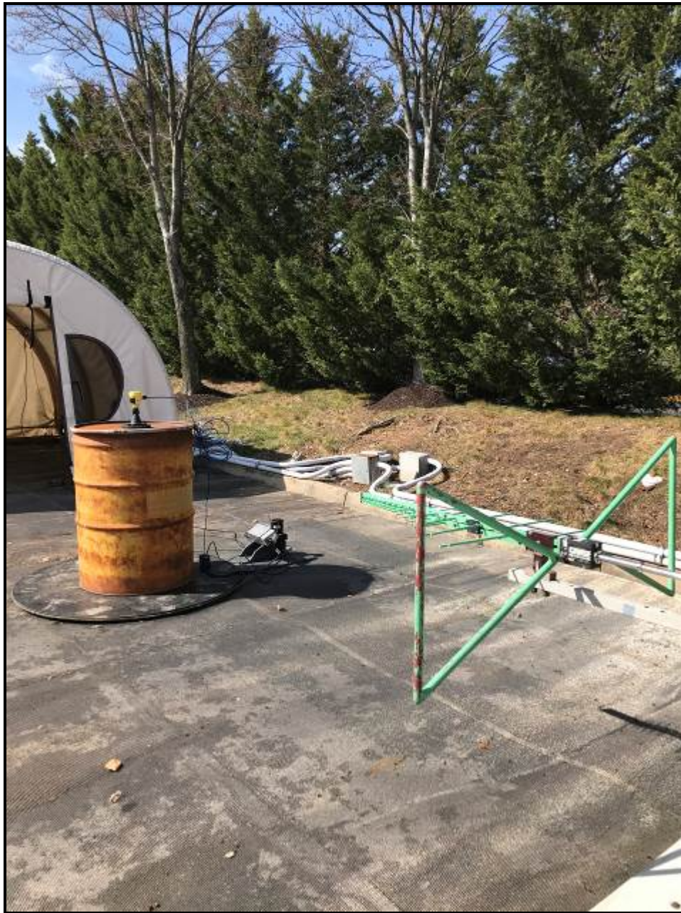
Photograph 12: Radiated Emissions – TC #1; Steel Container
