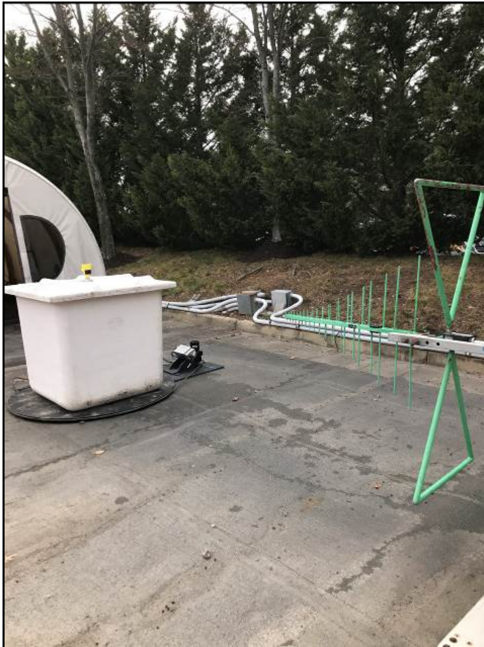
Photograph 16: Radiated Emissions – TC #2; Fiberglass Container
