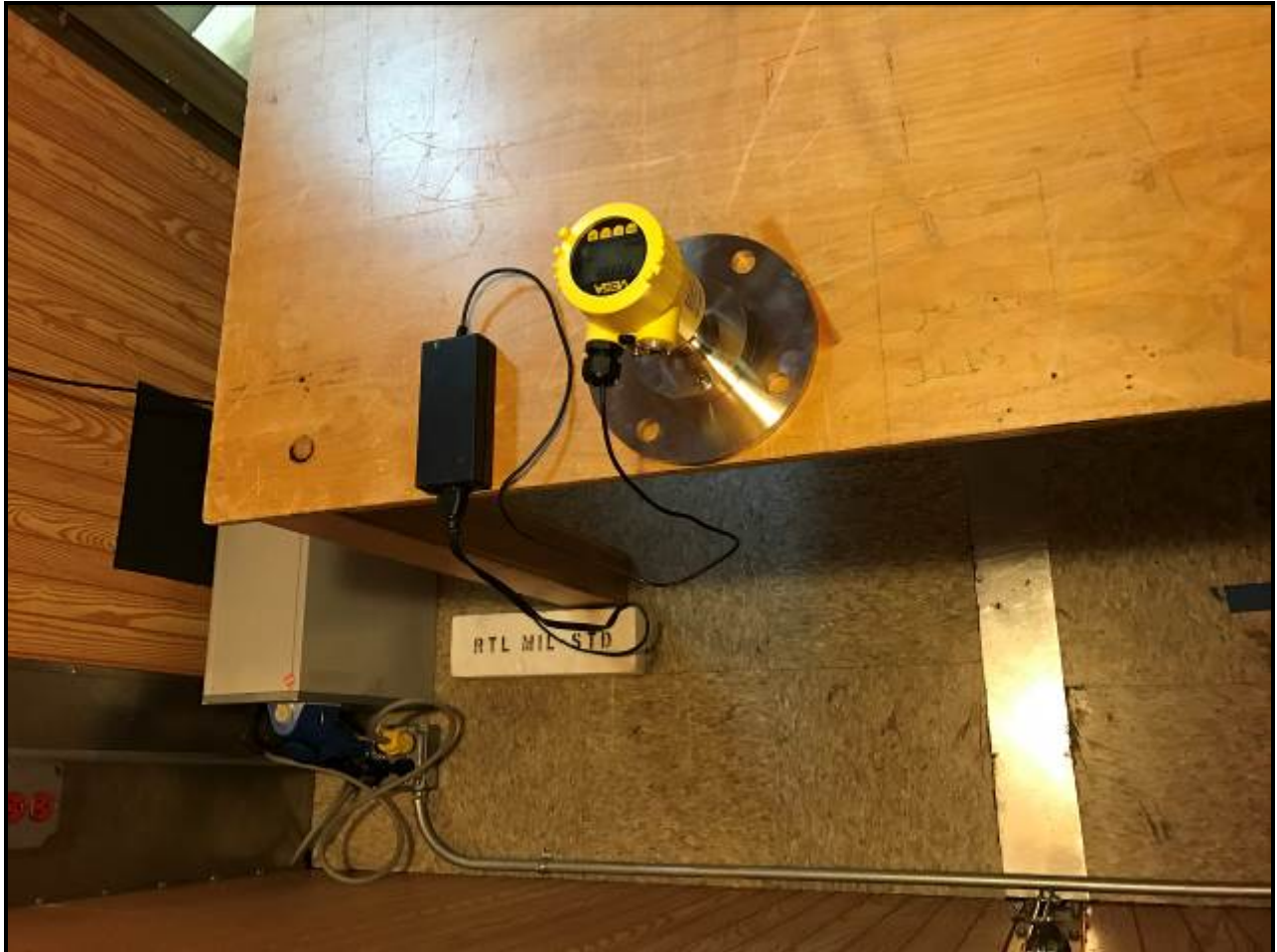
Photograph 8: AC Conducted Emissions - Rear View – TC #2
