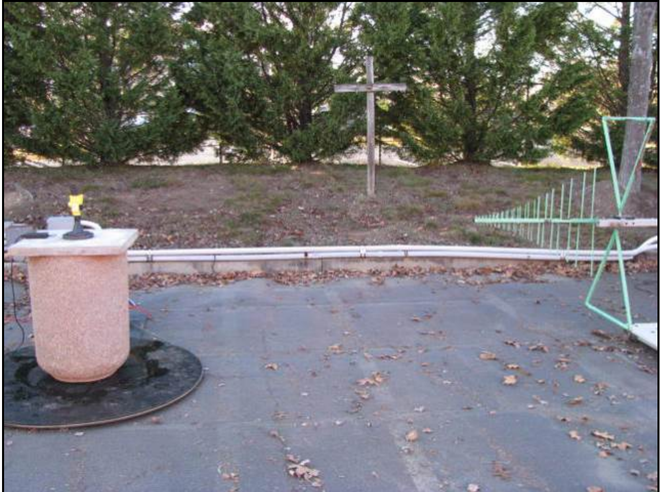
Photograph 11: Radiated Emissions – TC #1; Concrete Container
