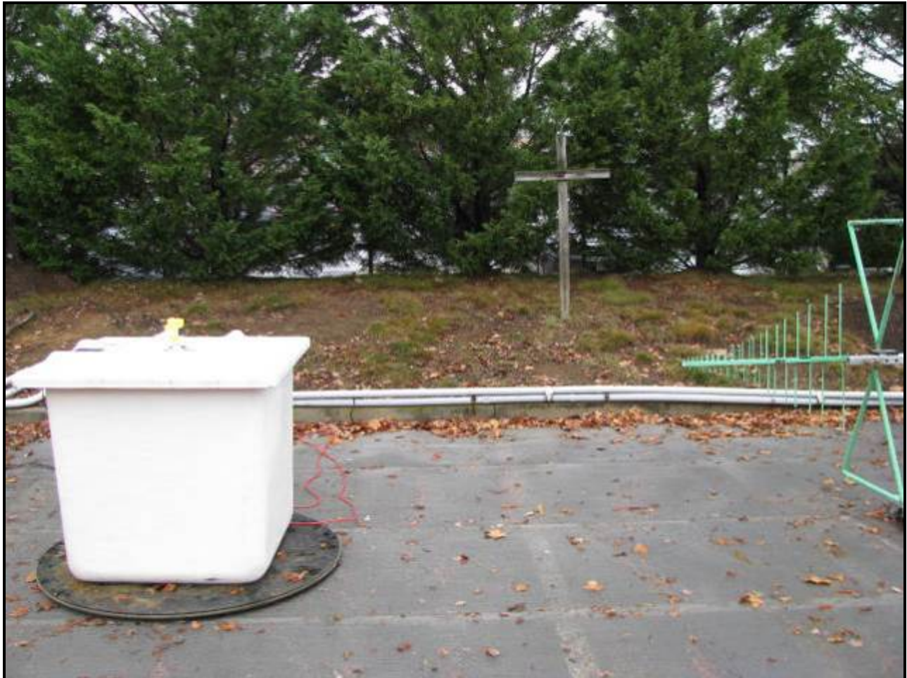
Photograph 16: Radiated Emissions – TC #2; Fiberglass Container
