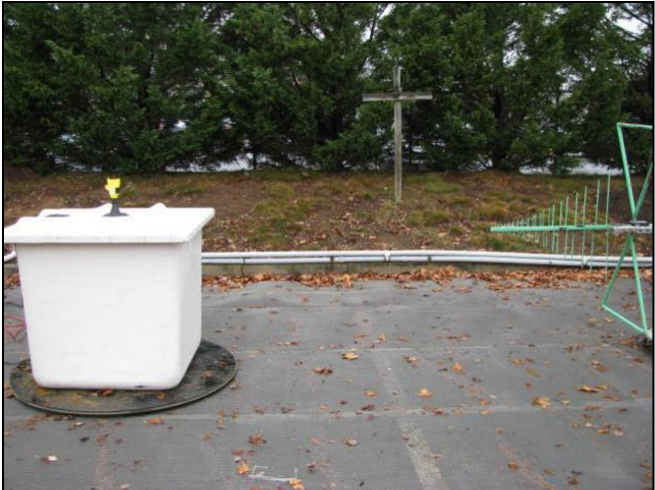
Photograph 13: Radiated Emissions – TC #1; Fiberglass Container
