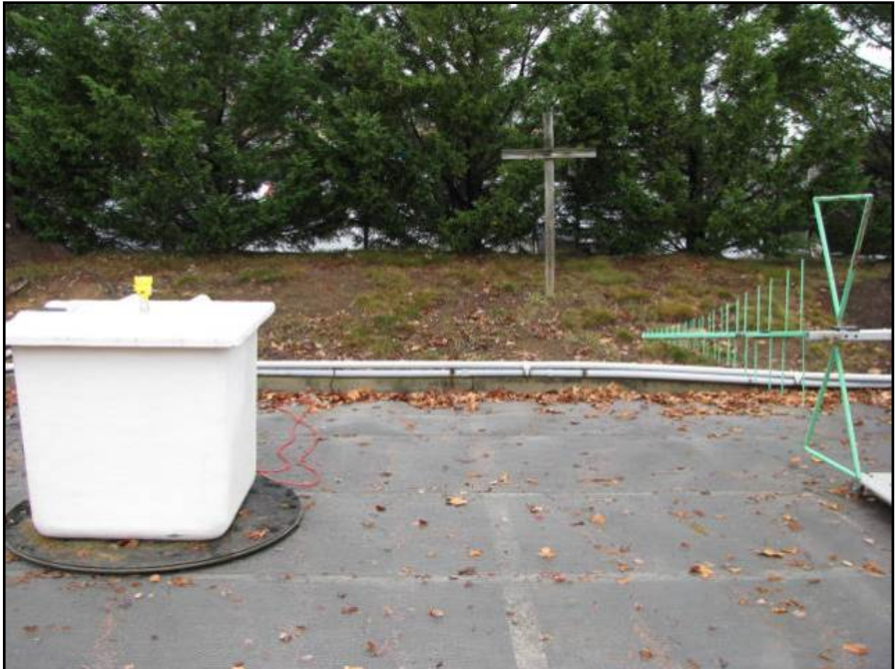
Photograph 19: Radiated Emissions – TC #3; Fiberglass Container
