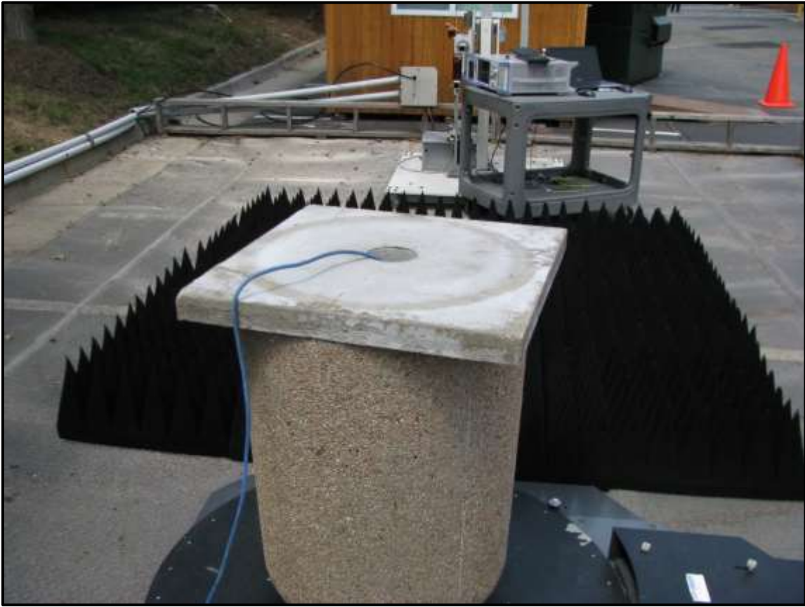
Photograph 19: Radiated Emissions – TC #1 Swivel; Concrete Container, Front View
