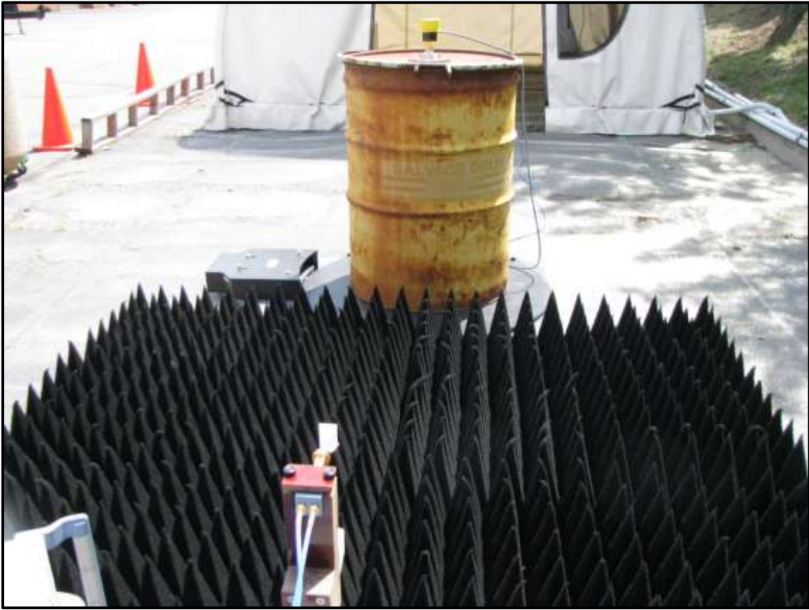
Photograph 8: Radiated Emissions – TC #1; Steel Container, Front View
