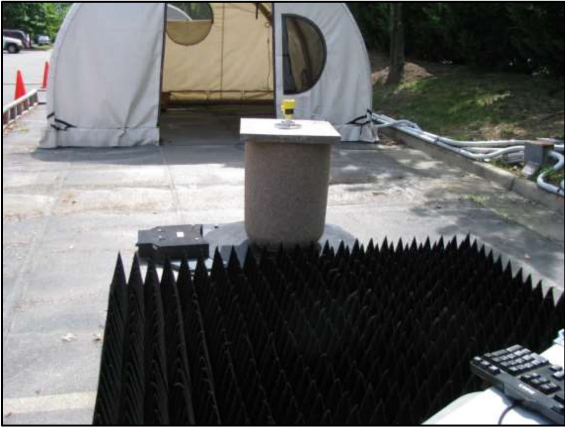
Photograph 15: Radiated Emissions – TC #2; Concrete Container, Rear View
