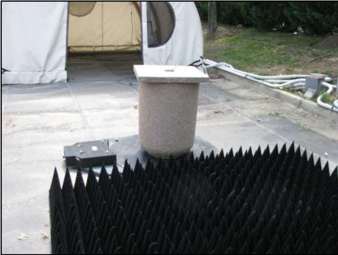
Photograph 20: Radiated Emissions – TC #1 Swivel; Concrete Container, Rear View
