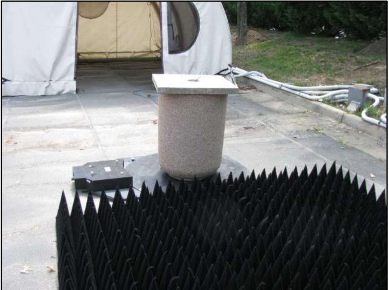
Photograph 24: Radiated Emissions – TC #2 Swivel; Concrete Container, Rear View
