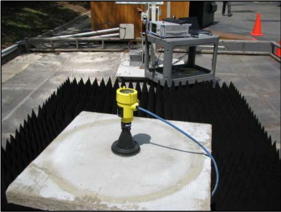
Photograph 10: Radiated Emissions – TC #1; Concrete Container, Front View
