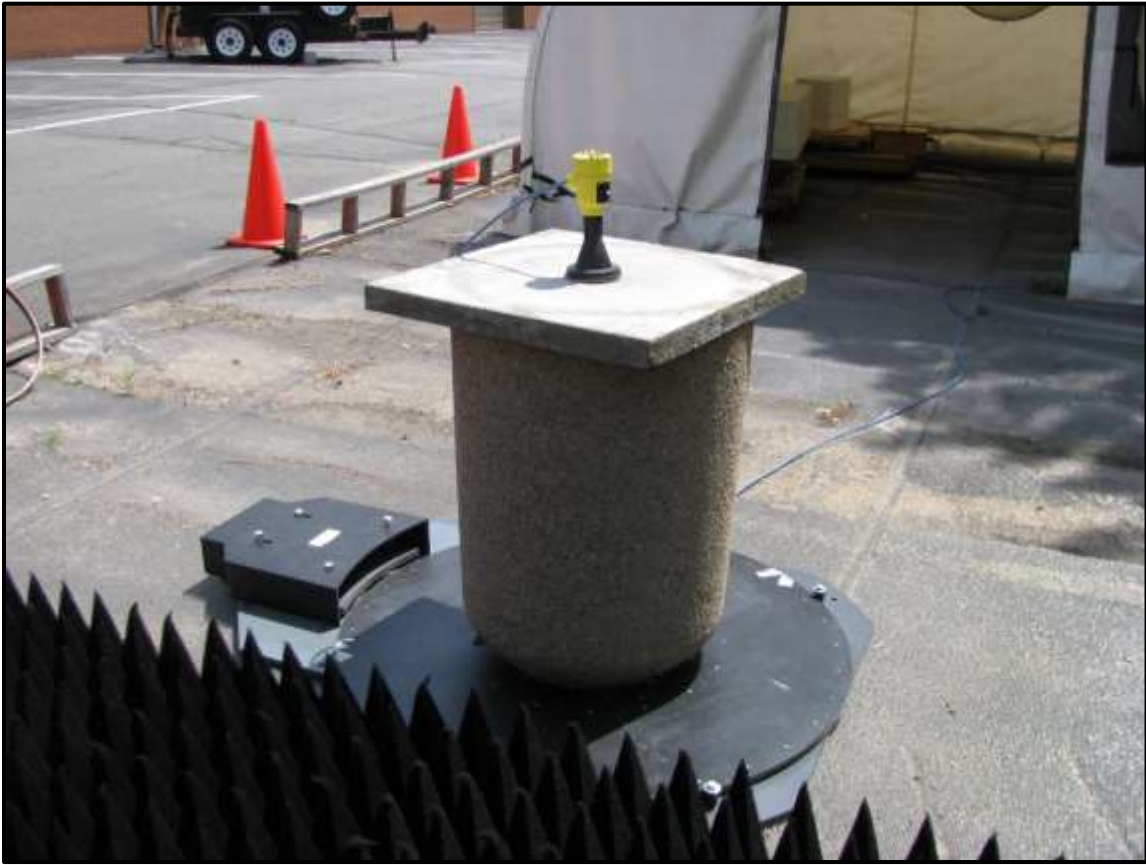
Photograph 11: Radiated Emissions – TC #1; Concrete Container, Rear View
