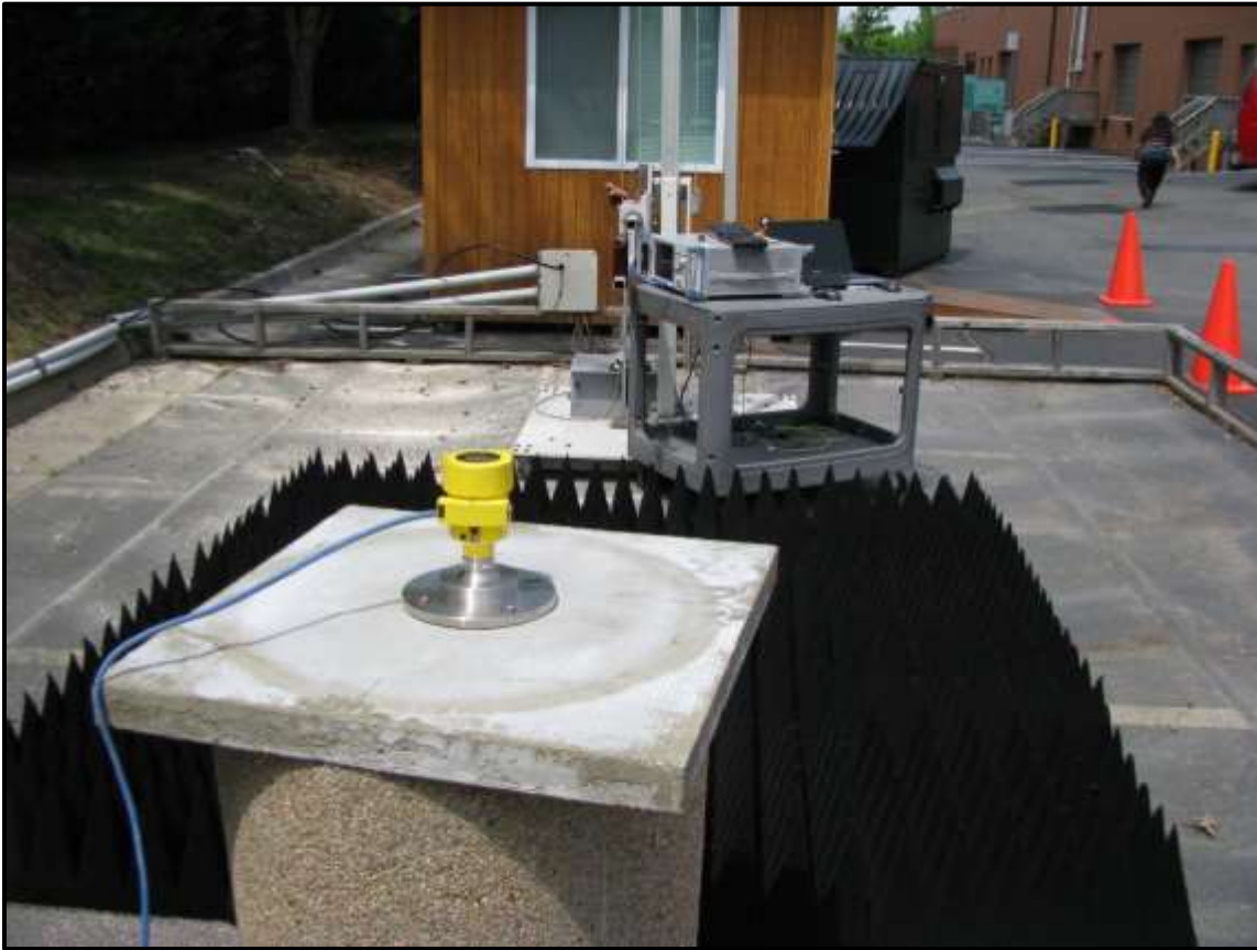
Photograph 14: Radiated Emissions – TC #2; Concrete Container, Front View
