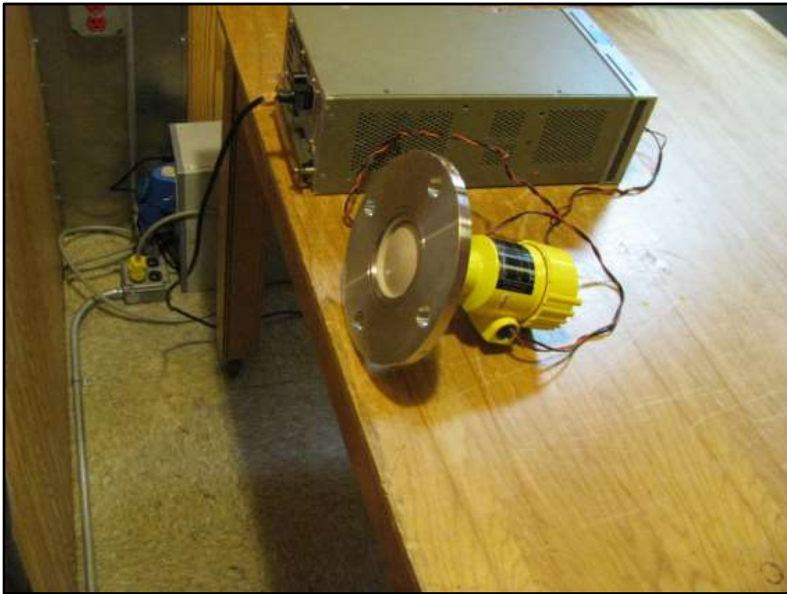
Photograph 6: Conducted Emissions – TC #2, Front View
