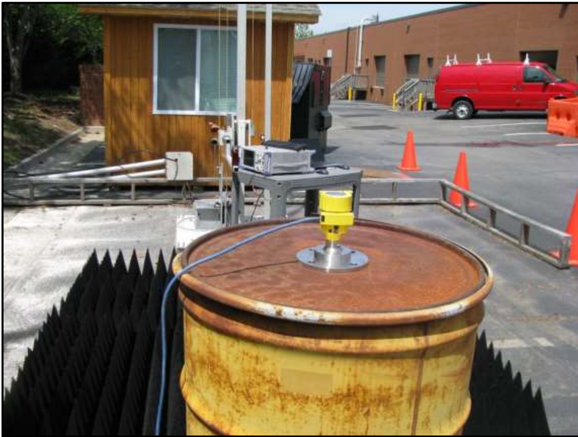
Photograph 13: Radiated Emissions – TC #2; Steel Container, Rear View
