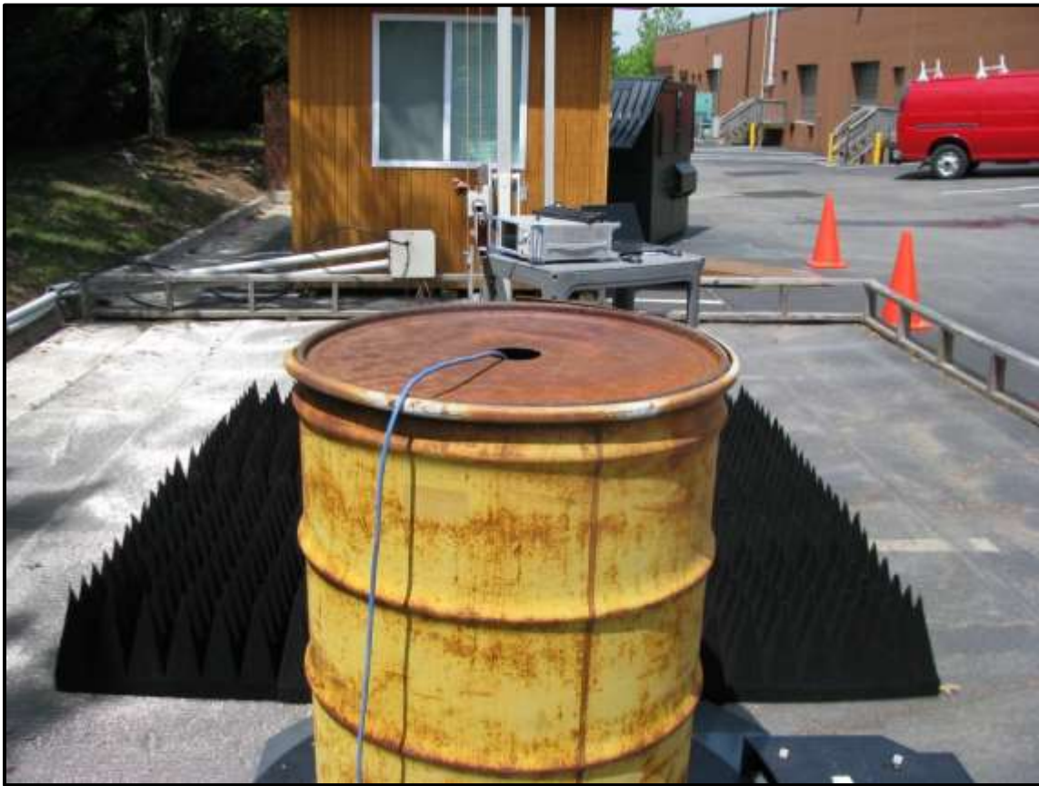
Photograph 21: Radiated Emissions – TC #2 Swivel; Steel Container, Front View
