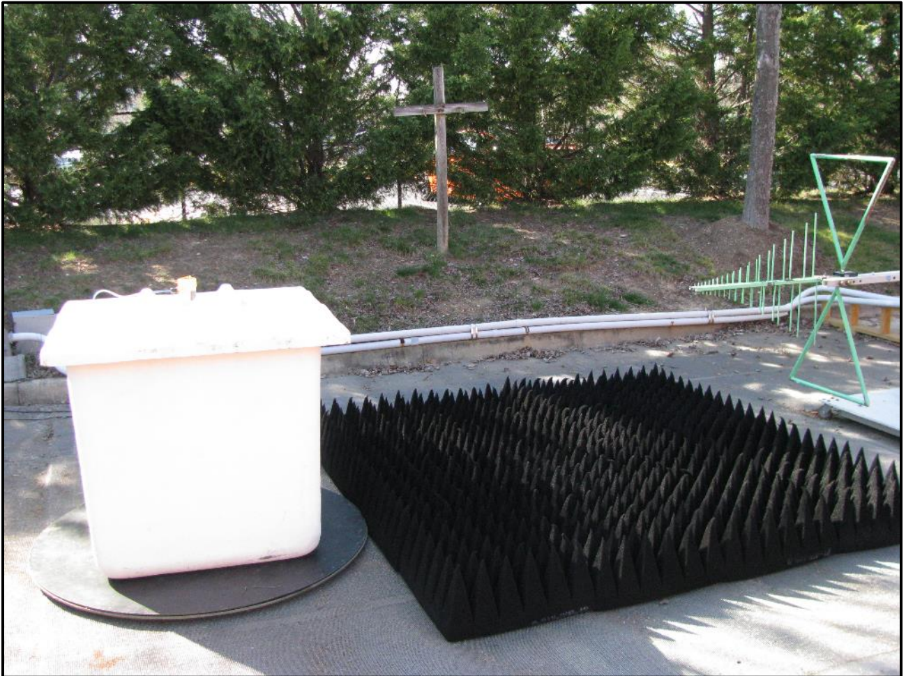
Photograph 55: Radiated Emissions – TC #4; Fiberglass Container, Front View
