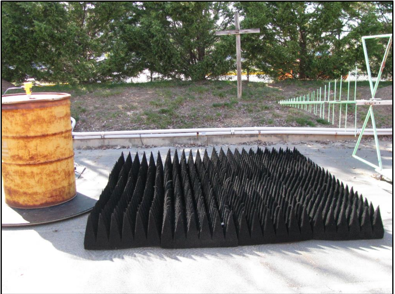
Photograph 24: Radiated Emissions – TC #6; Steel Container, Rear View
