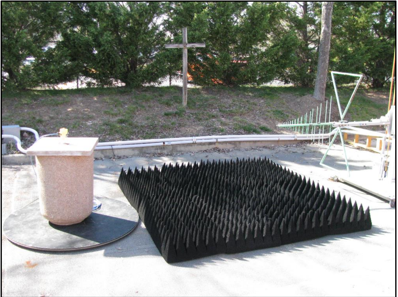
Photograph 34: Radiated Emissions – TC #2; Concrete Container, Rear View
