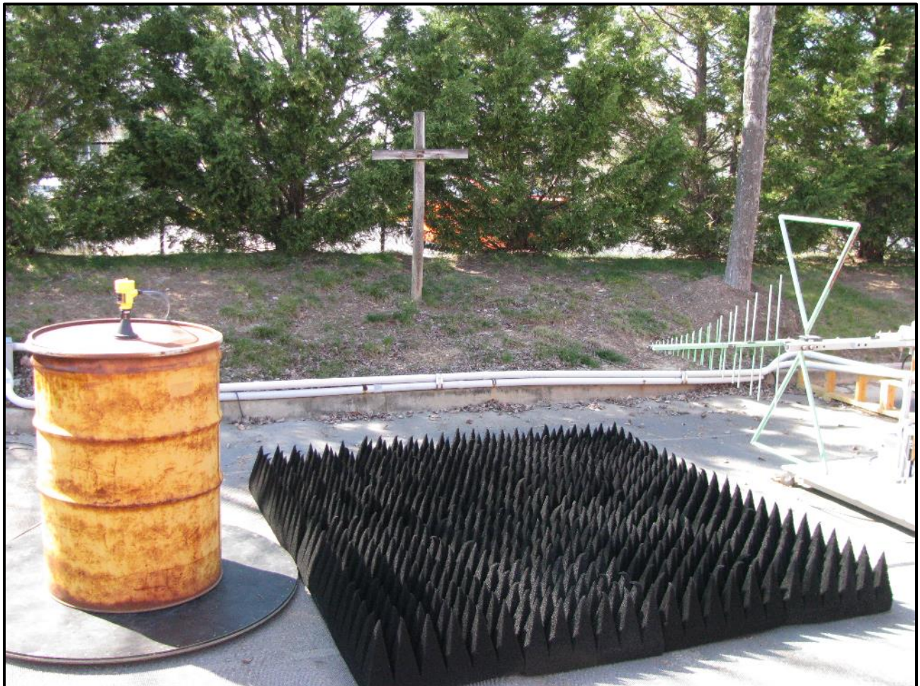
Photograph 14: Radiated Emissions – TC #1; Steel Container, Rear View
