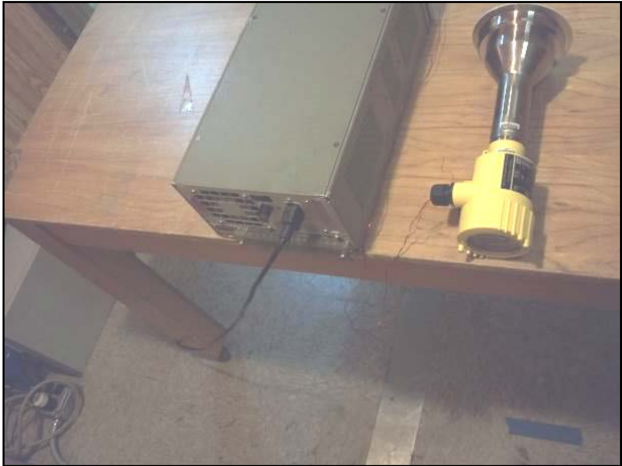
Photograph 8: AC Conducted Emissions - Rear View (TC #10)
