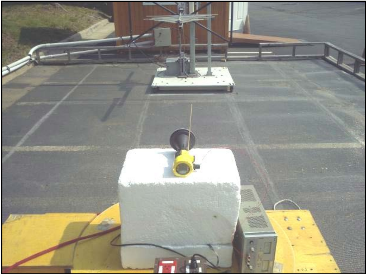
Photograph 6: Radiated Emissions – Rear View (TC #10)
