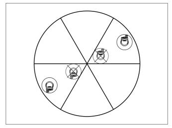
Fig. 17: Installation of VEGAPULS 68 in multiple chamber silos
