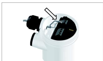
Insert the cable into the sensor through the cable entry
