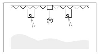
Fig. 14: Radar sensors on traverse crane
