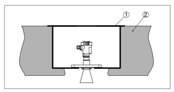
Fig. 16: Mounting of the instrument in an subsurface enclosure
