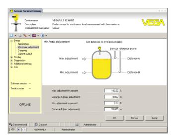
Fig. 32: Example of a DTM view
