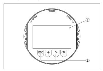
Fig. 29: Indicating and adjustment elements
