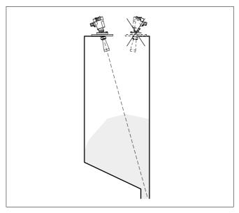
Fig. 18: Orientation of VEGAPULS 68 for emptying in the silo center
