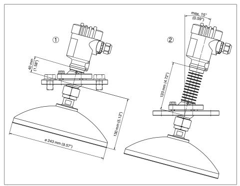
Fig. 44: Radar sensor with parabolic antenna and swivelling holder
