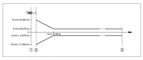
Fig. 34: Deviation under reference conditions
