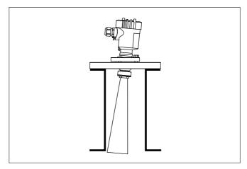
Fig. 8: Distance between antenna and socket
