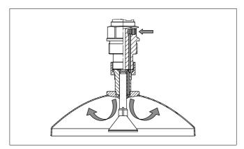
Fig. 20: Purging air connection with parabolic antenna
