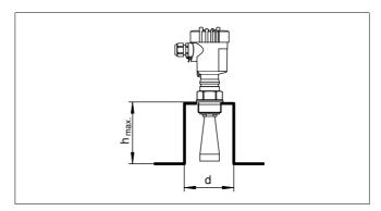
Fig. 9: Deviating socket dimensions
