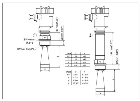
Fig. 41: Radar sensor with horn antenna in threaded version
