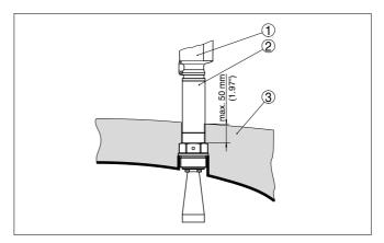
Fig. 15: Mounting of the instrument with insulated vessels.
