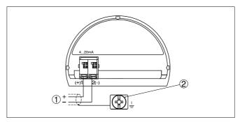
Fig. 26: Connection compartment double chamber housing Ex d
