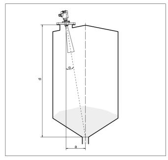
Fig. 11: Proposal for installation after orientation VEGAPULS 68
