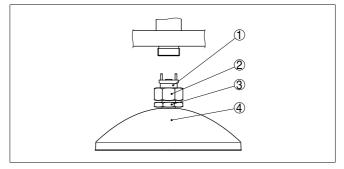
Fig. 3: Dismounting, parabolic antenna
