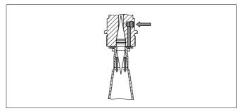
Fig. 19: Purging air connection with horn antenna
