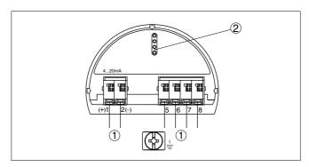
Fig. 23: Electronics compartment, double chamber housing
