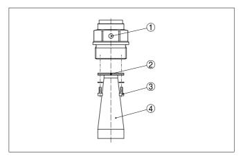
Fig. 2: Dismounting of the horn antenna
