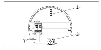
Fig. 24: Connection compartment, double chamber housing
