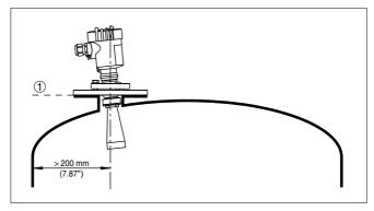
Fig. 5: Mounting of the radar sensor on round vessel tops
