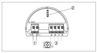
Fig. 25: Electronics compartment, double chamber housing
