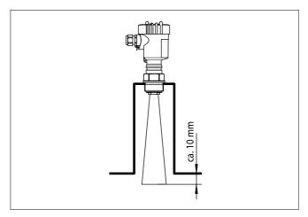
Fig. 7: Recommended socket mounting
