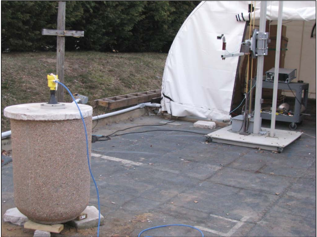
Photograph 30: 80mm Plastic Antenna Rear View Concrete Tank
