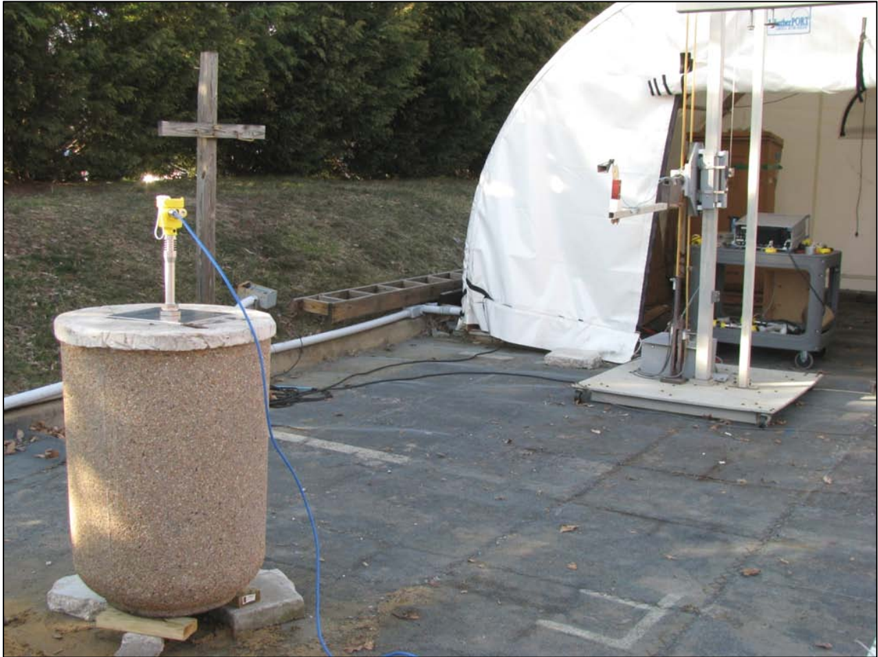
Photograph 33: 1/2" Standpipe Antenna Front View Concrete Tank
