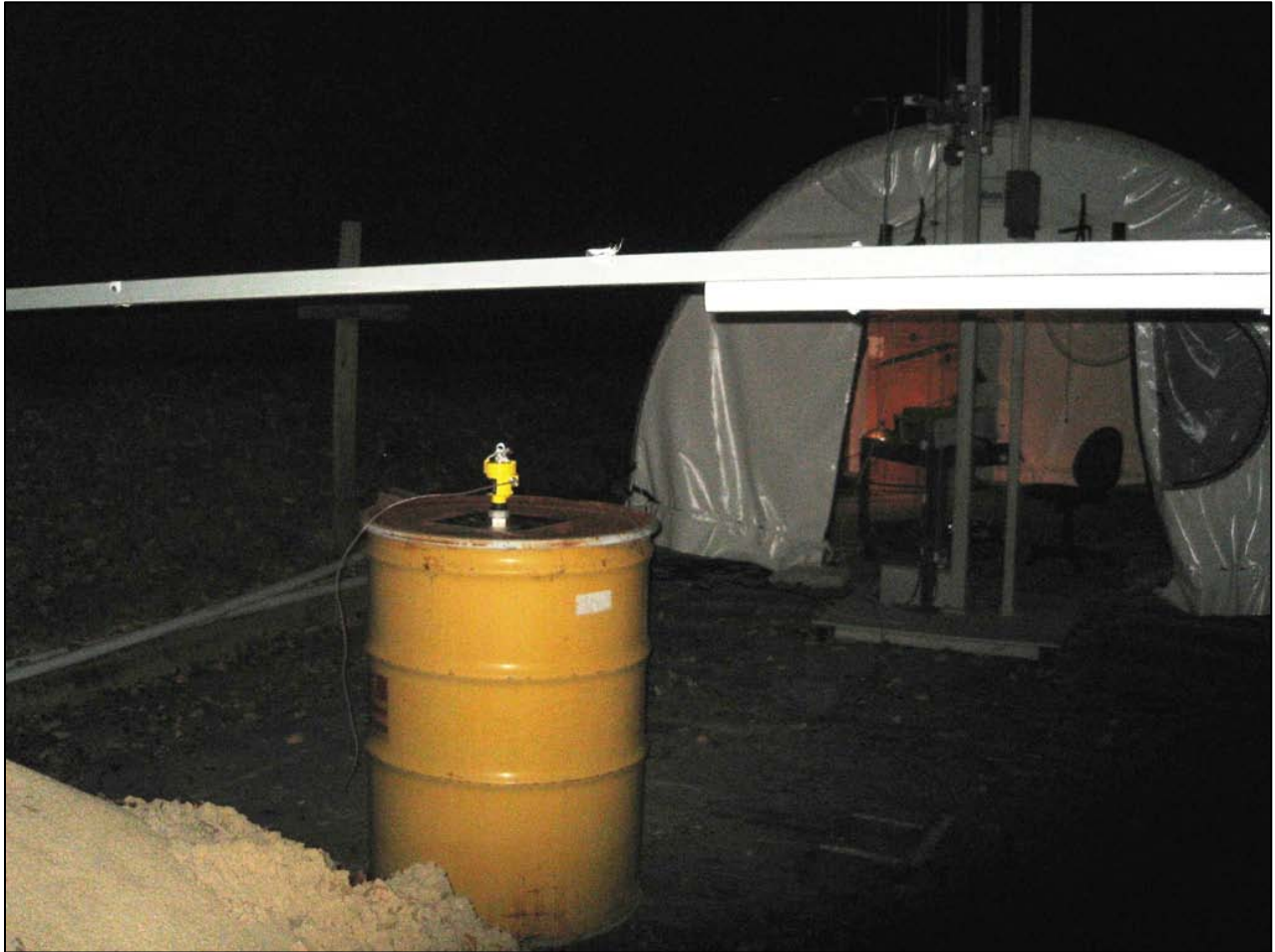
Photograph 15: 1/2" Stub Antenna Front View Metal Tank
