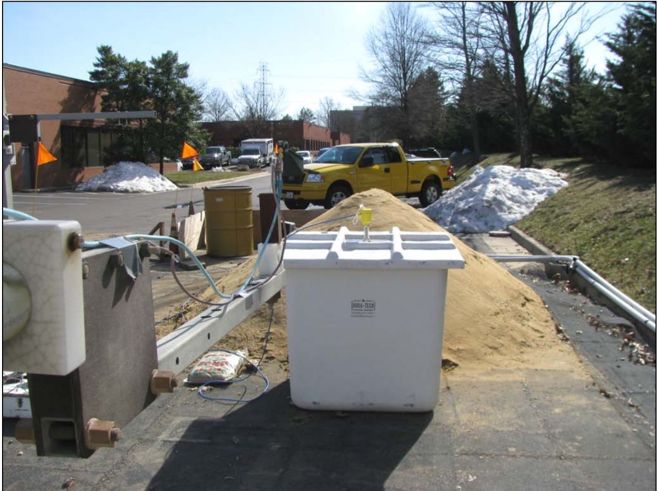
Photograph 35: 245mm Antenna Front View Fiberglass Tank
