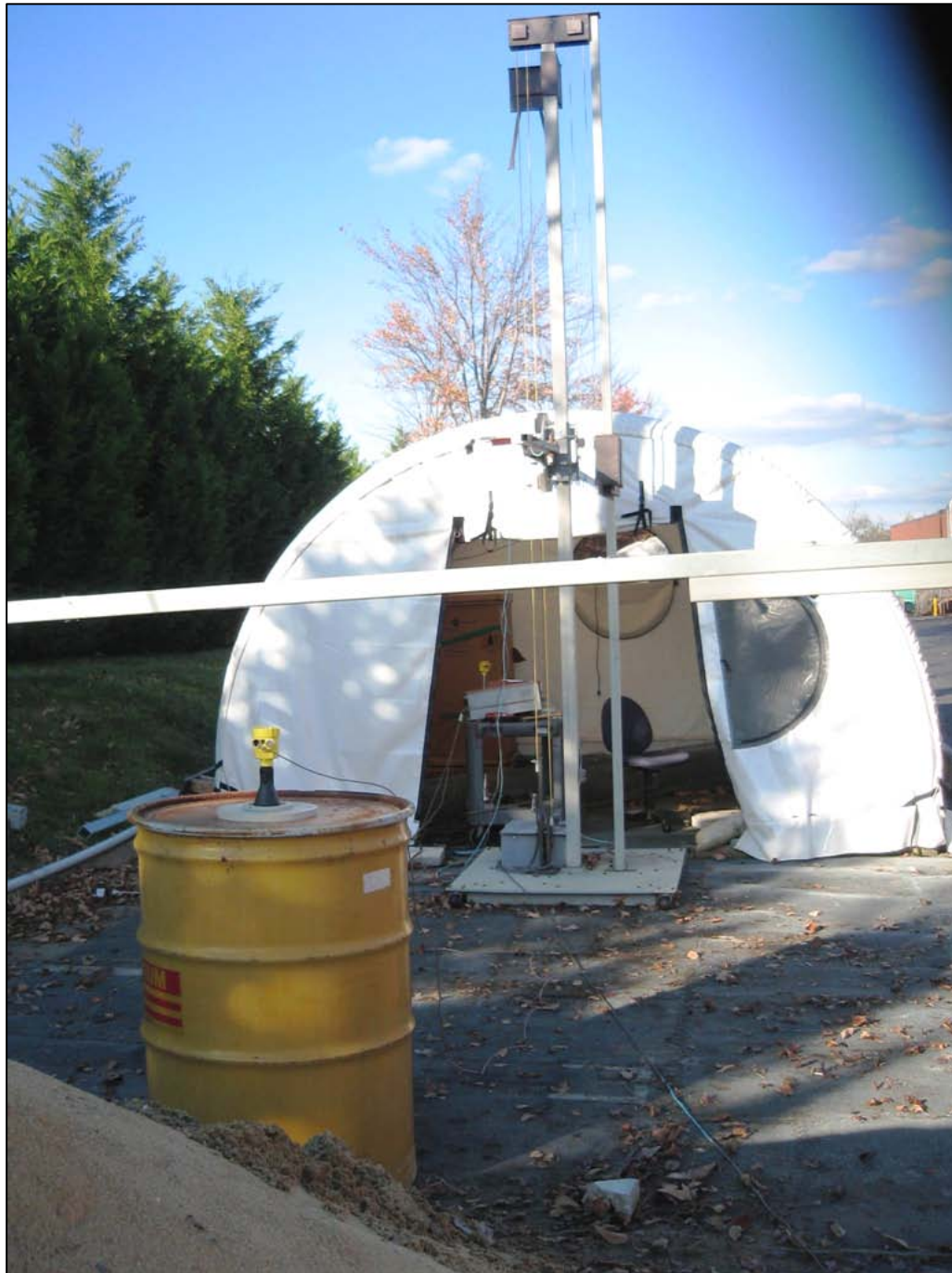
Photograph 14: 80mm Plastic Horn Antenna Rear View Metal Tank
