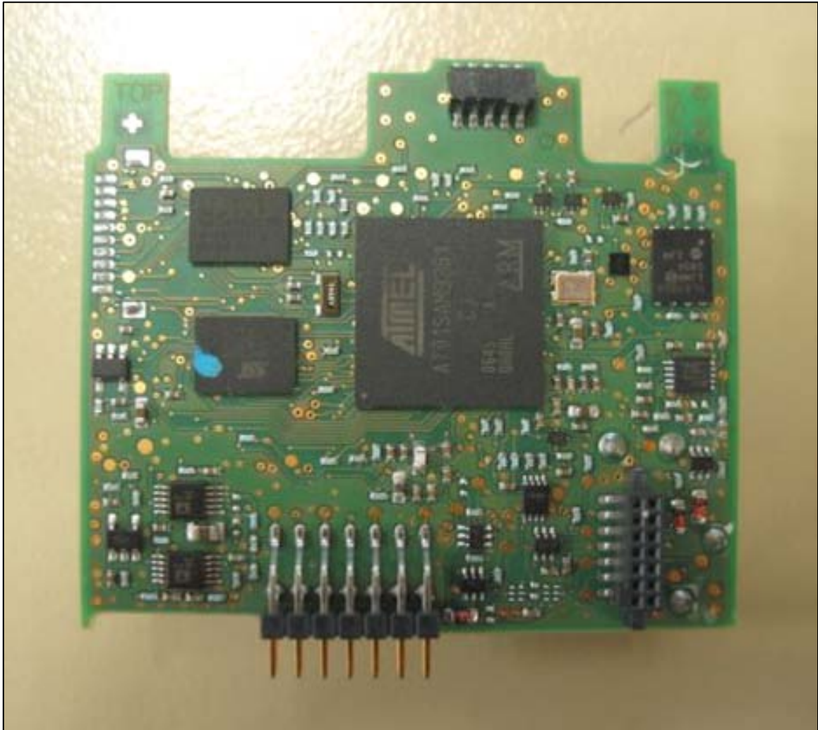
PHOTOGRAPH 5: CPU BOARD (COMPONENT SIDE)
