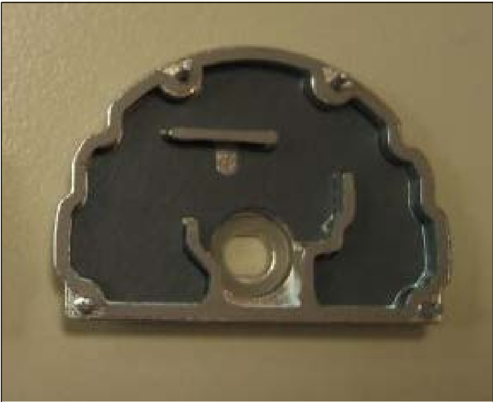
PHOTOGRAPH 12: MICROWAVE SHIELD INSIDE
