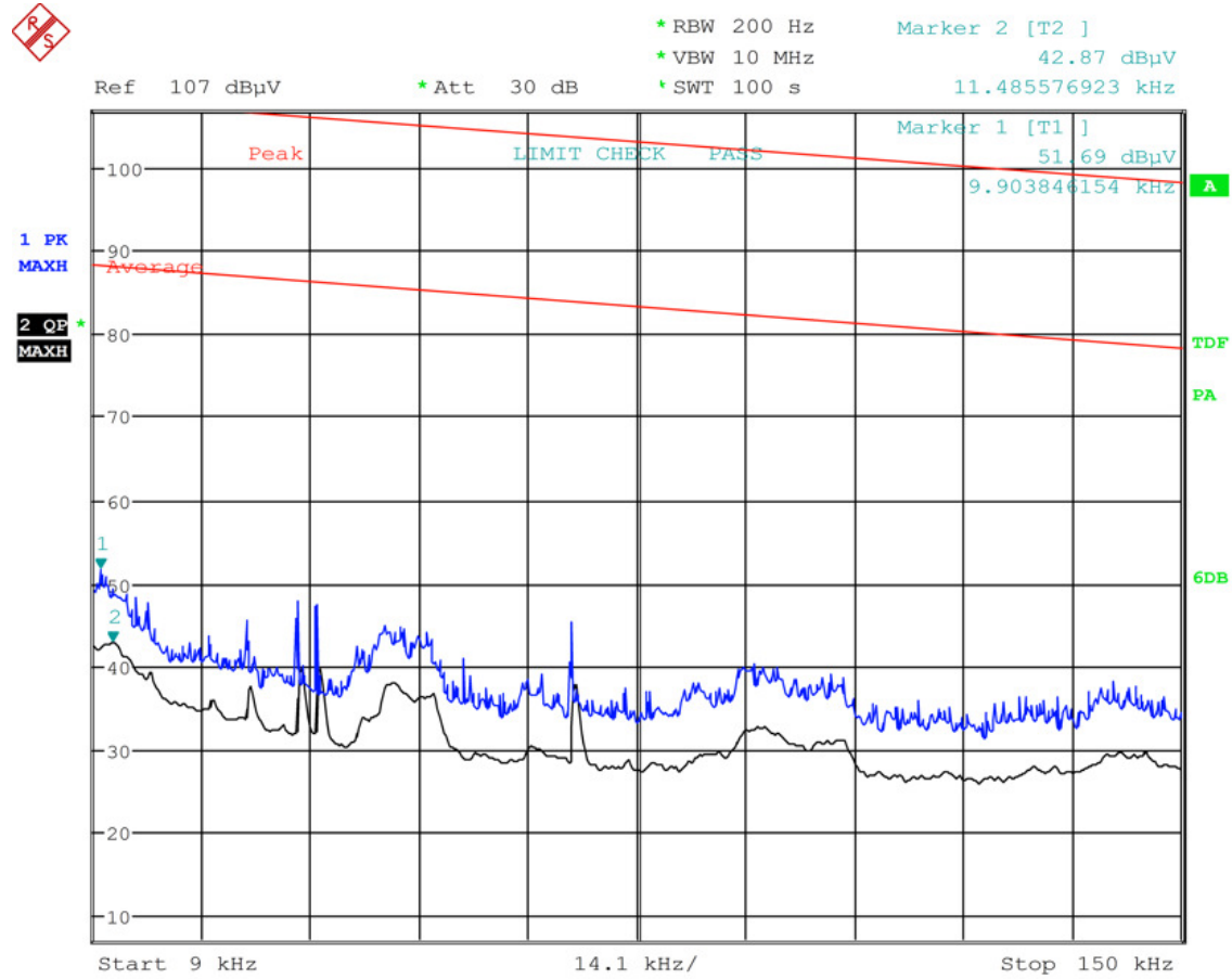
Plot 6-42: Radiated Emissions Transmit – 9 kHz – 150 kHz Horizontal Peak/Average
