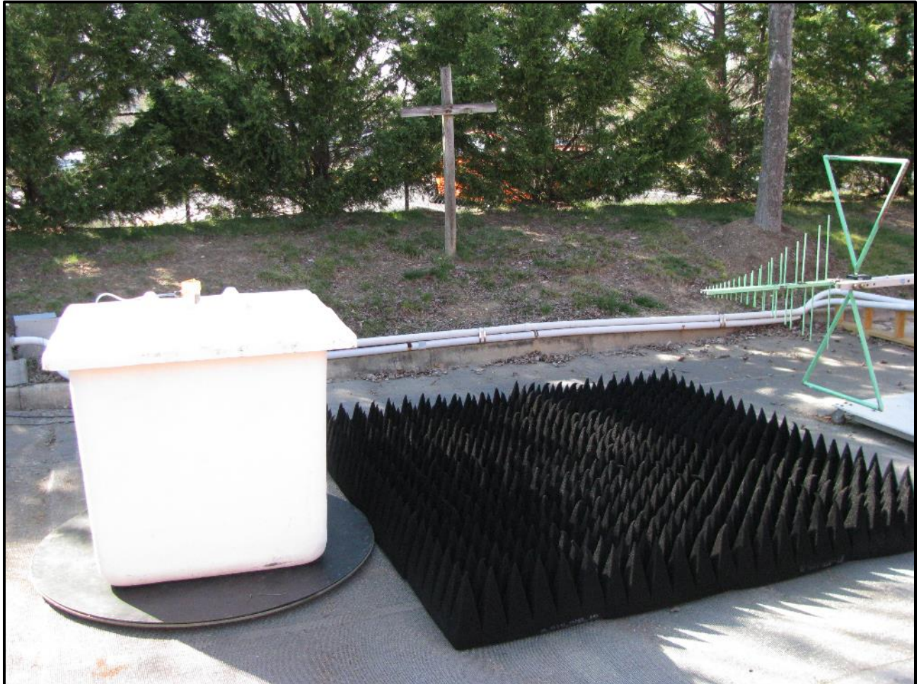
Photograph 55: Radiated Emissions – TC #4; Fiberglass Container, Front View
