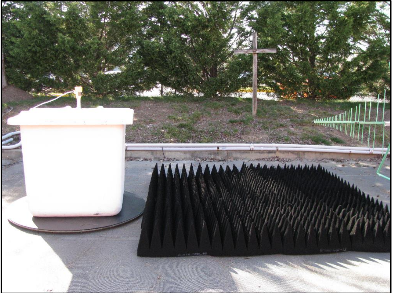
Photograph 62: Radiated Emissions – TC #7; Fiberglass Container, Rear View
