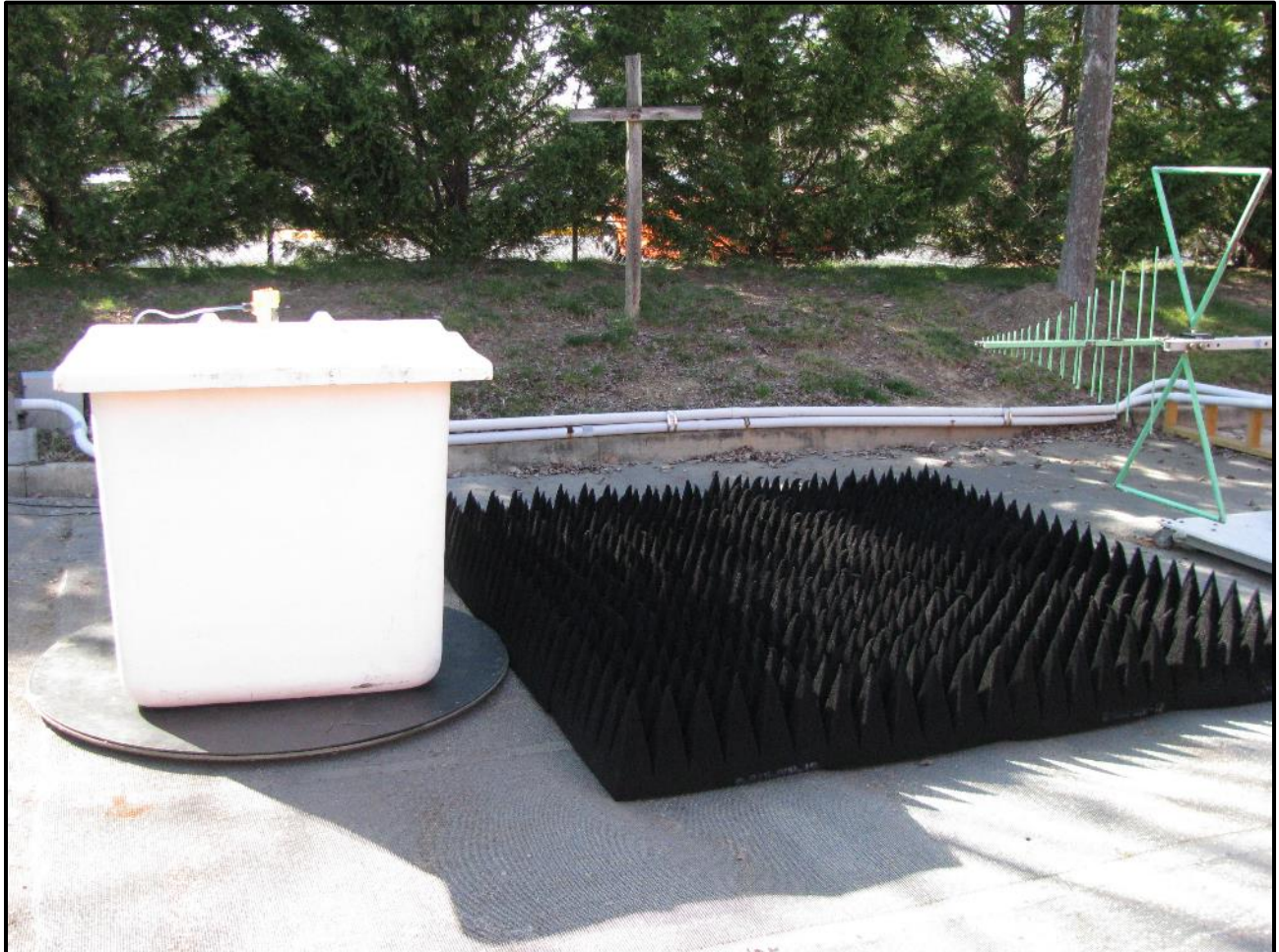
Photograph 56: Radiated Emissions – TC #4; Fiberglass Container, Rear View
