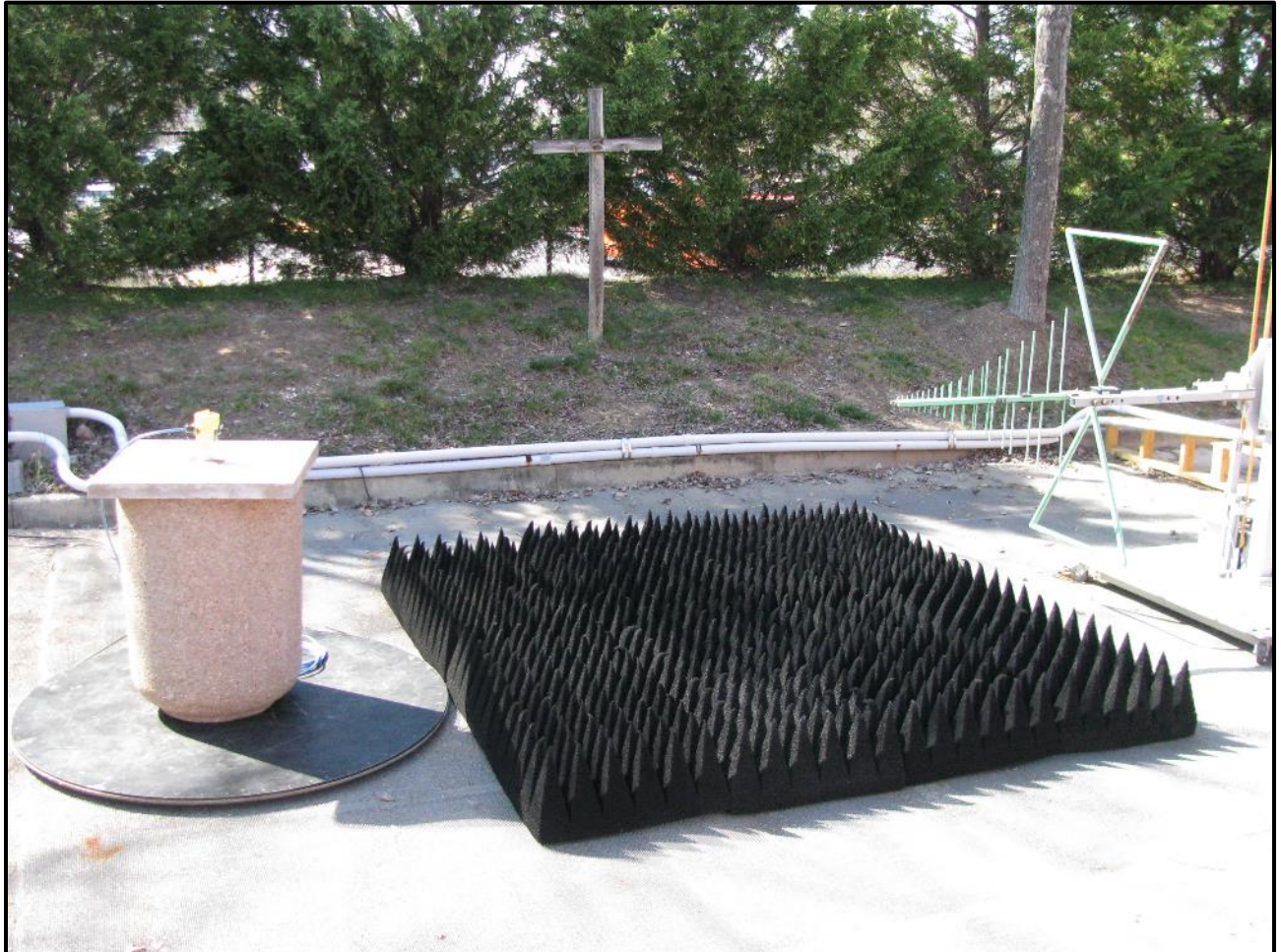
Photograph 42: Radiated Emissions – TC #6; Concrete Container, Rear View
