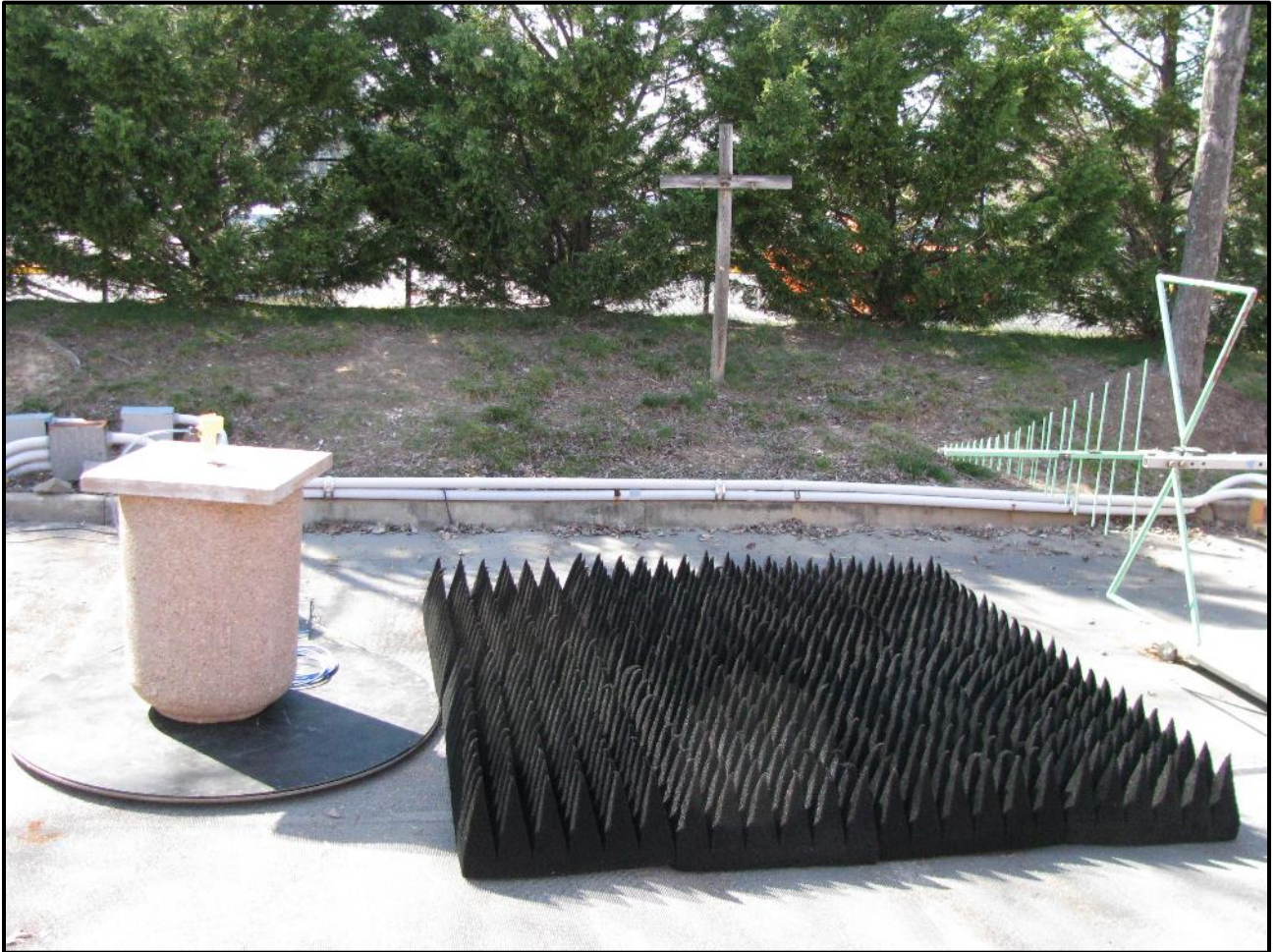
Photograph 39: Radiated Emissions – TC #5; Concrete Container, Front View
