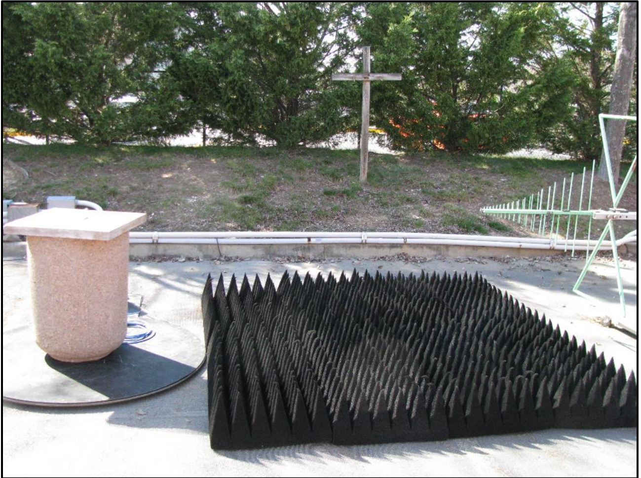
Photograph 45: Radiated Emissions – TC #8; Concrete Container, Front View
