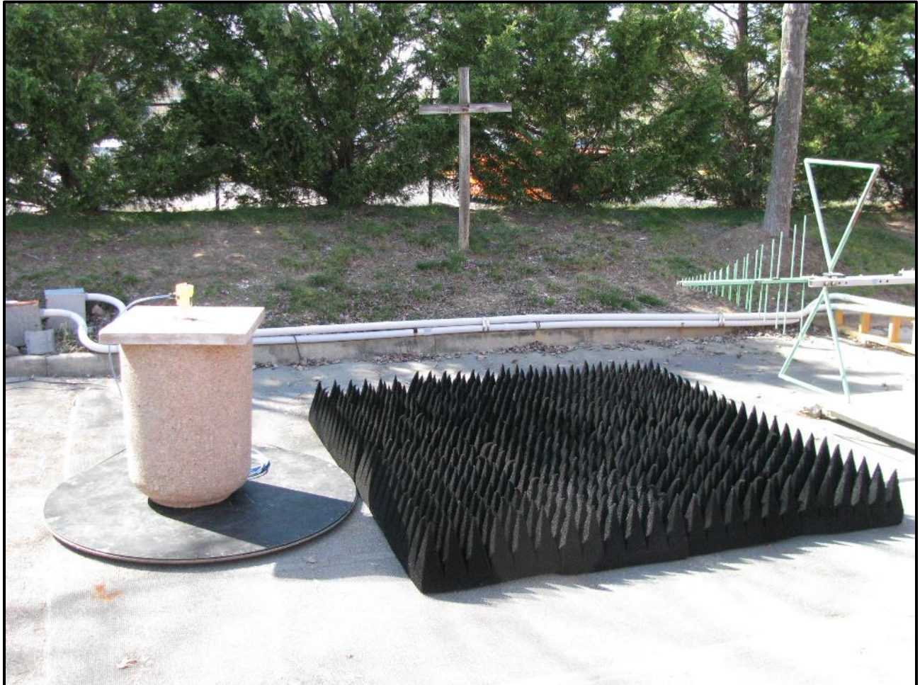
Photograph 33: Radiated Emissions – TC #2; Concrete Container, Front View
