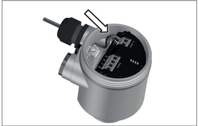
Fig. 22: Connection steps 5 and 6 - Single chamber housing
