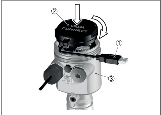
Fig. 38: Connection of the PC directly to the sensor via the interface adapter
