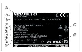
Fig. 1: Structure of the type label (example)
