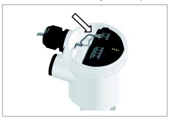
5 Insert the cable into the sensor through the cable entry
