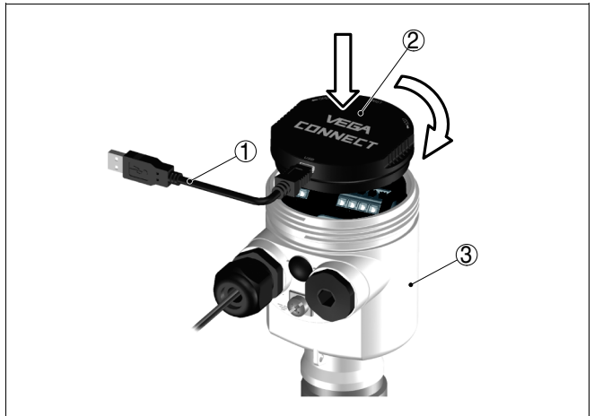
Fig. 23: Connection of the PC directly to the sensor via the interface adapter
