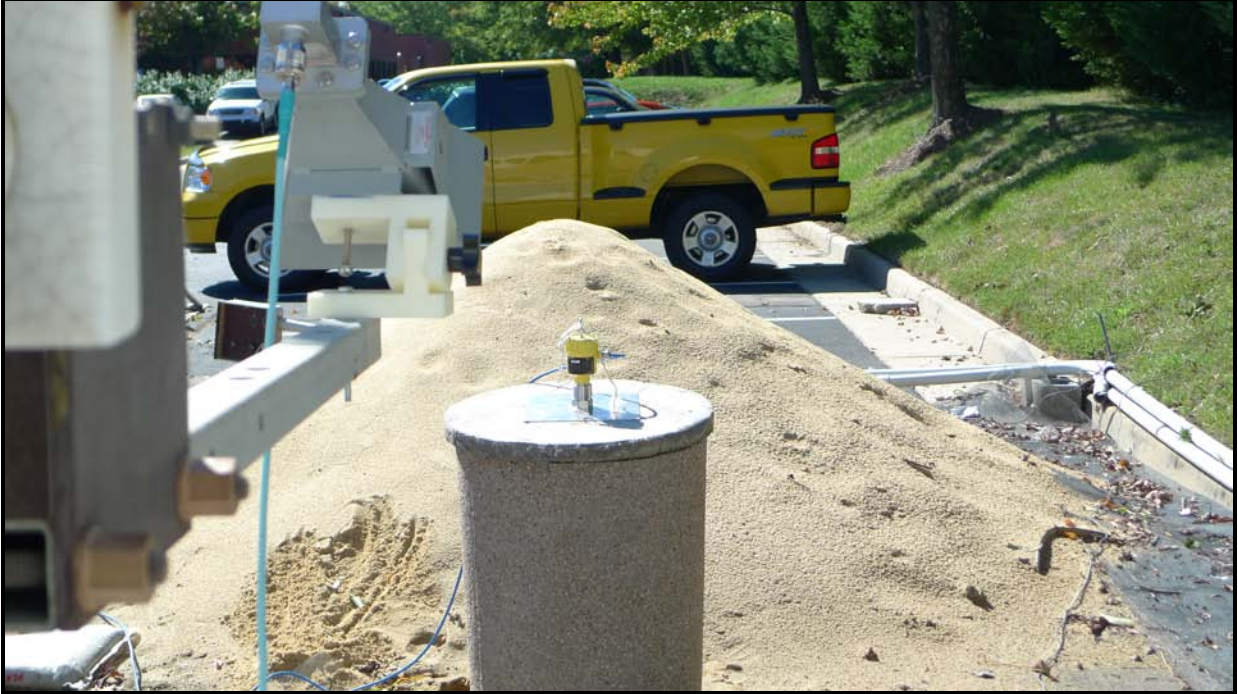
Photograph 11: 10" Horn Antenna Front View Concrete Tank
