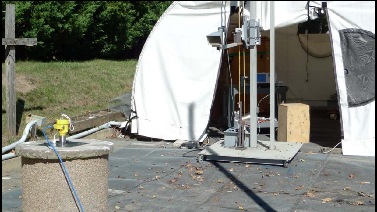
Photograph 12: 10" Horn Antenna Rear View Concrete Tank
