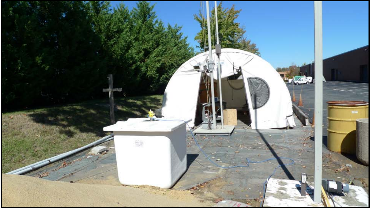
Photograph 22: 4" Horn Antenna Rear View Fiberglass Tank
