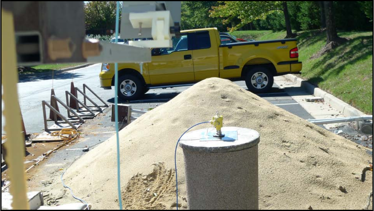
Photograph 13: 4" Horn Antenna Front View Concrete Tank
