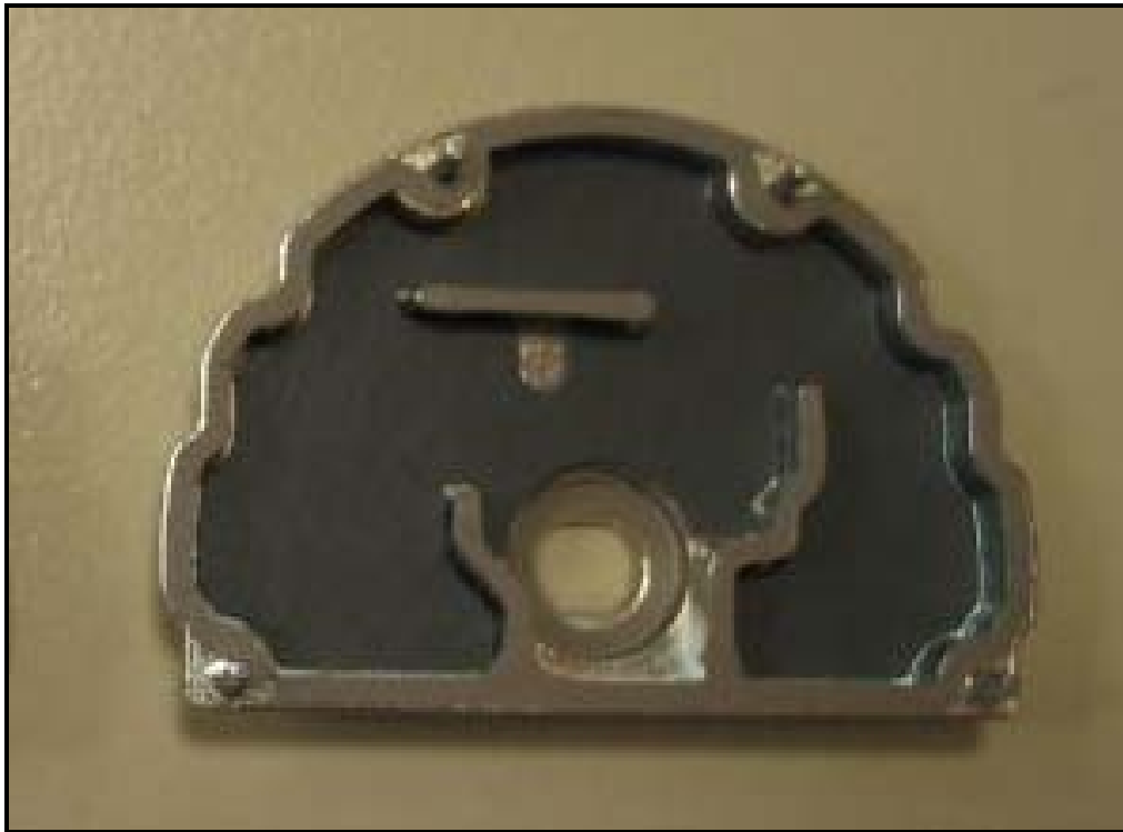
Photograph 13: Microwave Board (Shielding Side)
