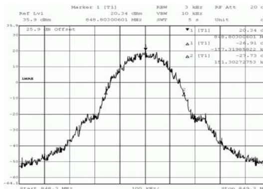
Title: bandwidth measurement Comment A1: DE1015003, E2008850, 26dB bandwidth, channel 251 (848.8MHz) Date: 15.JUL.2014 23:24:45
