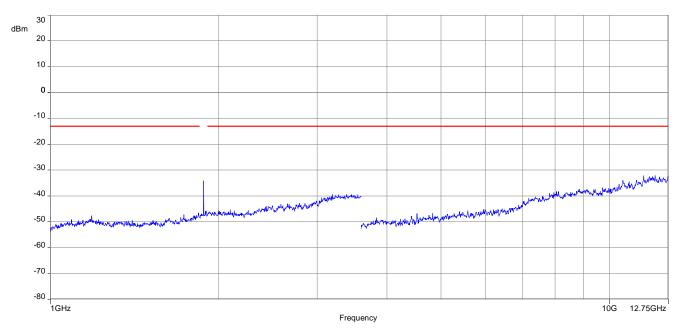
Carrier notched with 1.9 GHz rejection filter
