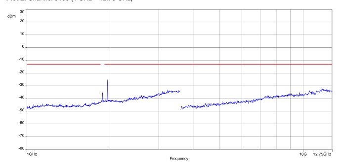
Carrier notched with 1.9 GHz rejection filter. Highest emission is the BS downlink signal.
