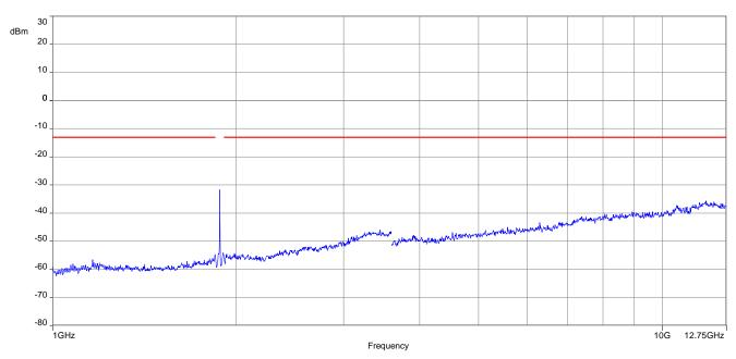
Carrier notched with 1.9 GHz rejection filter
