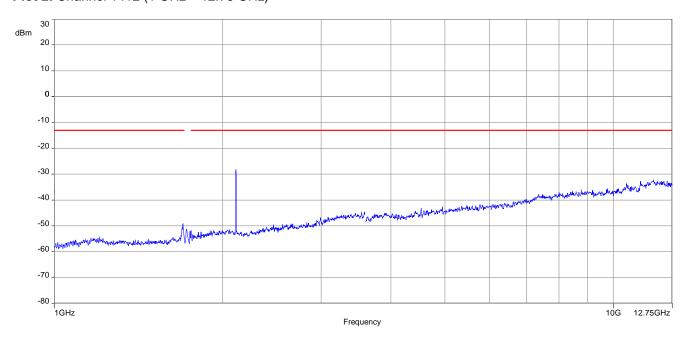
The carrier signal is notched with a band notch filter. Highest emission is the BS downlink signal.
