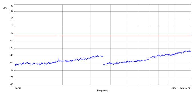
Carrier notched with 1.9 GHz rejection filter
