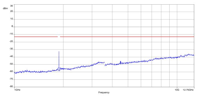
Carrier notched with 1.9 GHz rejection filter
