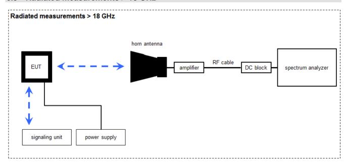
Measurement distance: horn antenna 25 cm
