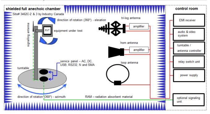
Measurement distance: tri-log antenna and horn antenna 3 meter; loop antenna 3 meter
