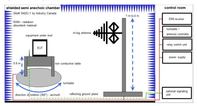
Measurement distance: tri-log antenna 10 meter
