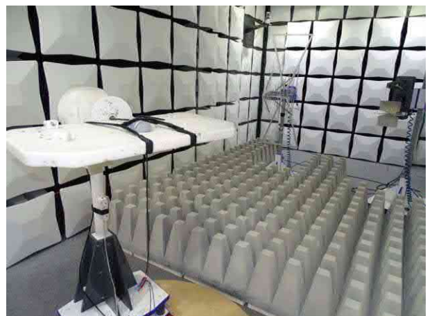
Photo 8-13: Test setup for radiated measurements (fully anechoic chamber, CFR 47 Part 15, Subpart B)
