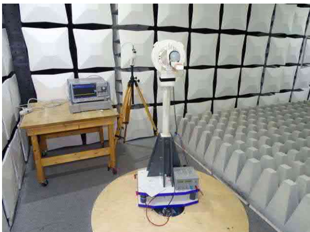
Photo 8-13: Test setup for radiated measurements (fully anechoic chamber, CFR 47 Part 15, Subpart B)
