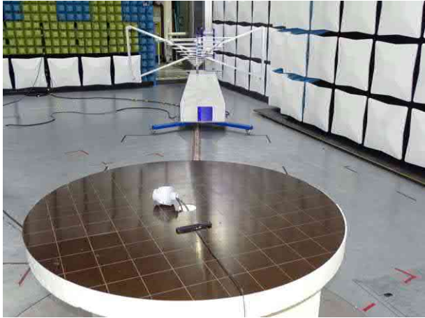
Photo 7: Test setup for radiated measurements (semi anechoic chamber, CFR 47 Part 15, Subpart C, §247)
