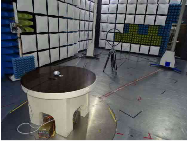
Photo 6: Test setup for radiated measurements (H-Field, CFR 47 Part 15, Subpart C, §247)
