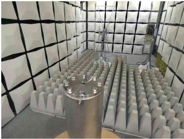
Photo 20: Test setup for radiated measurements (fully anechoic chamber, RSS-211, 5.3, inside the container)
