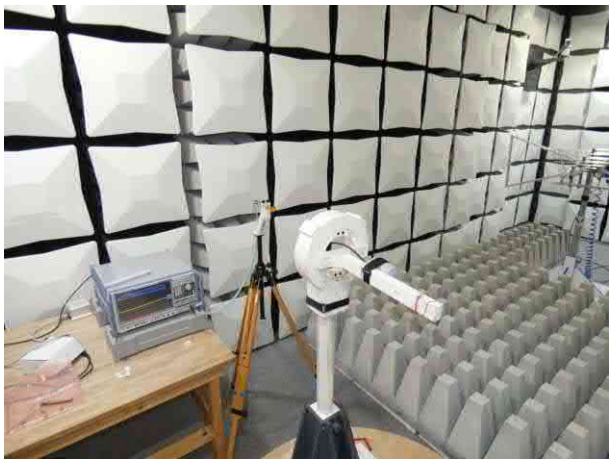
Photo 4-5: Test setup for radiated measurements (fully anechoic chamber, CFR 47 Part 15, Subpart C, §256)
