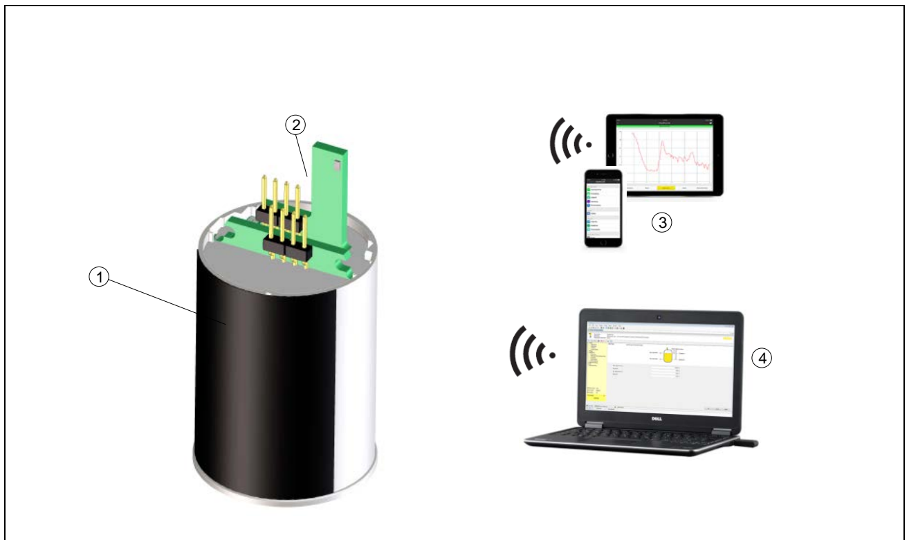
Fig. 8: Bluetooth connection to standard operating devices
