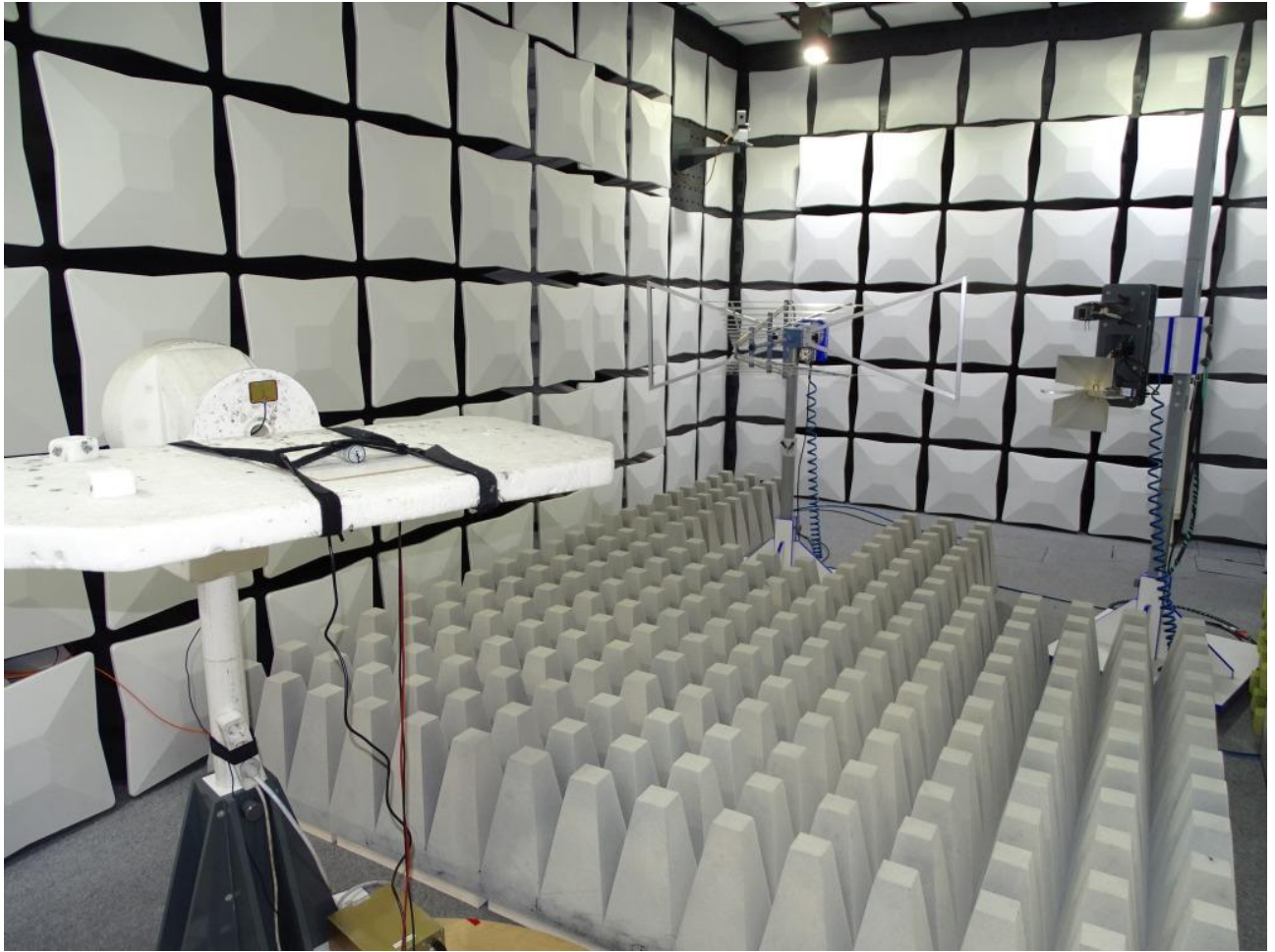
Photo 5: Test setup for radiated measurements (1 GHz – 24 GHz; FCC 15c247)
