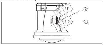
Fig. 14: Activate sensor by magnet
