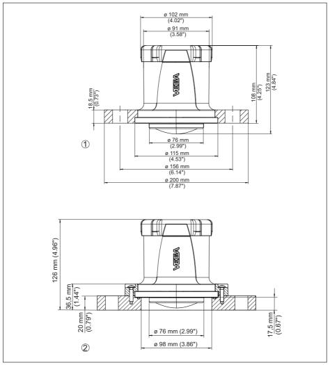
Fig. 22: Dimensions VEGAPULS Air 42
