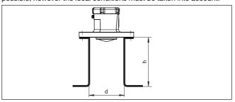
Fig. 9: Socket mounting with deviating socket dimensions
