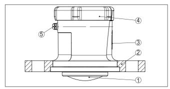
Fig. 1: Components of the VEGAPULS Air 42 sensor (Example version with compression flange DN 80)
