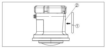
Fig. 13: Sensor activation via NFC technology
