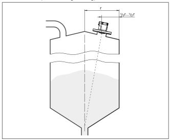
Fig. 11: Mounting position and orientation
