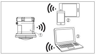
Fig. 3: Wireless connection to standard operating devices via Bluetooth
