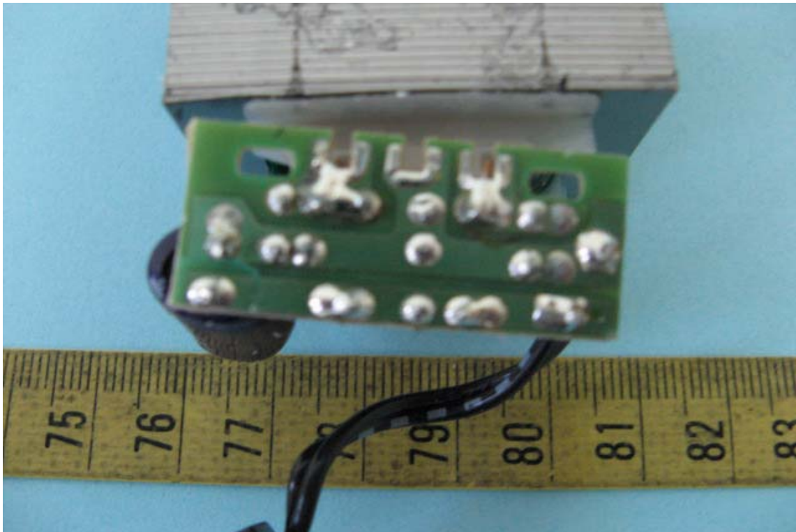
Solder View of Adaptor's PCB
