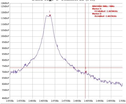
Brand / Model:傳世 / TTD-61RT(Monitor) Remark:CH22 SWT-2.5ms PK Horizontal Tested by:William
