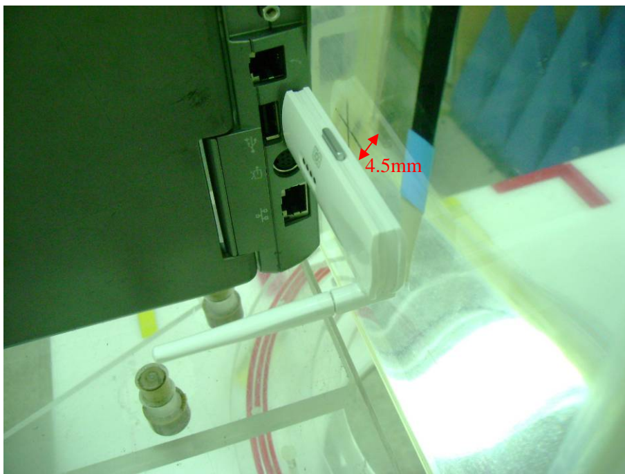
Figure 3: Bottom side of Laptop facing phantom touching (Horizontal-UP)-Zoom in
